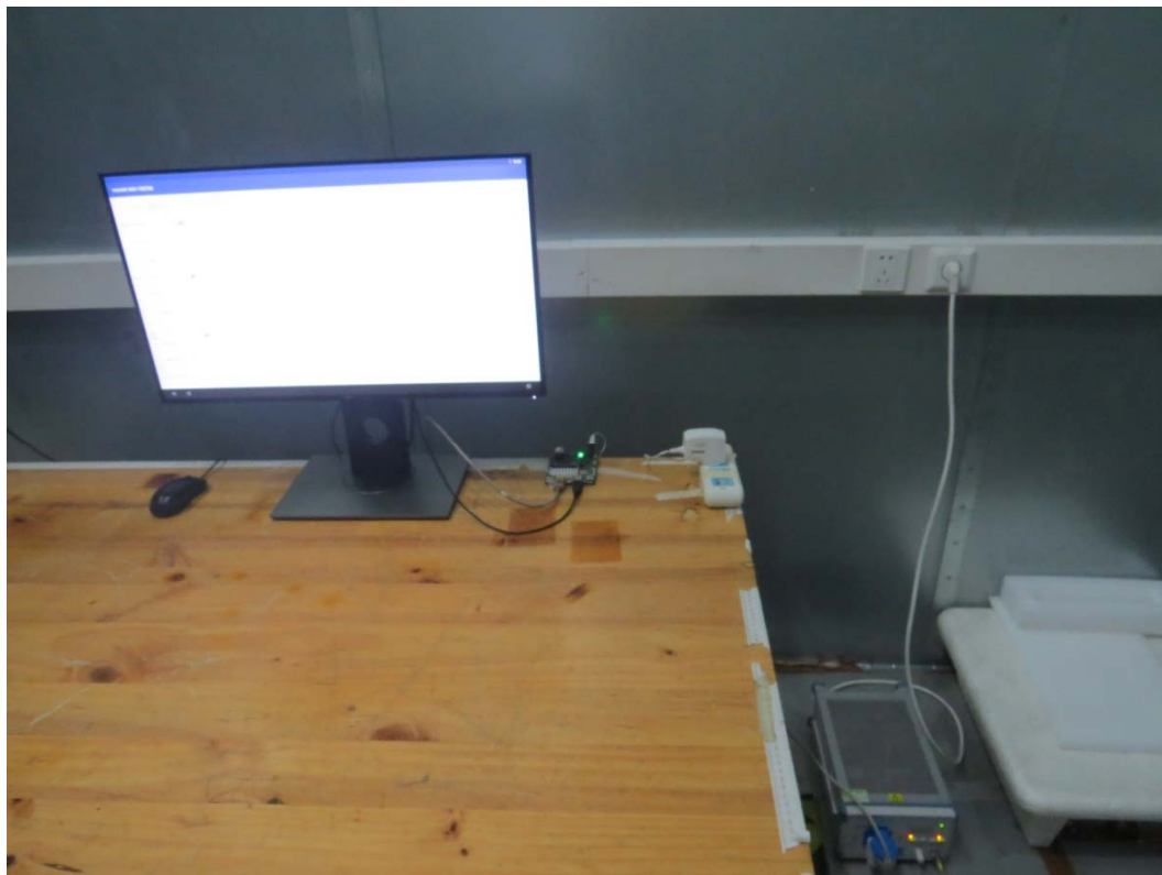
Picture 3 Conducted Emission Test Setup
