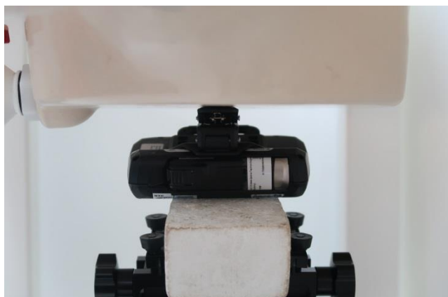
Hip Mount without keypad_Back with battery 2, Test Separation 0 mm
