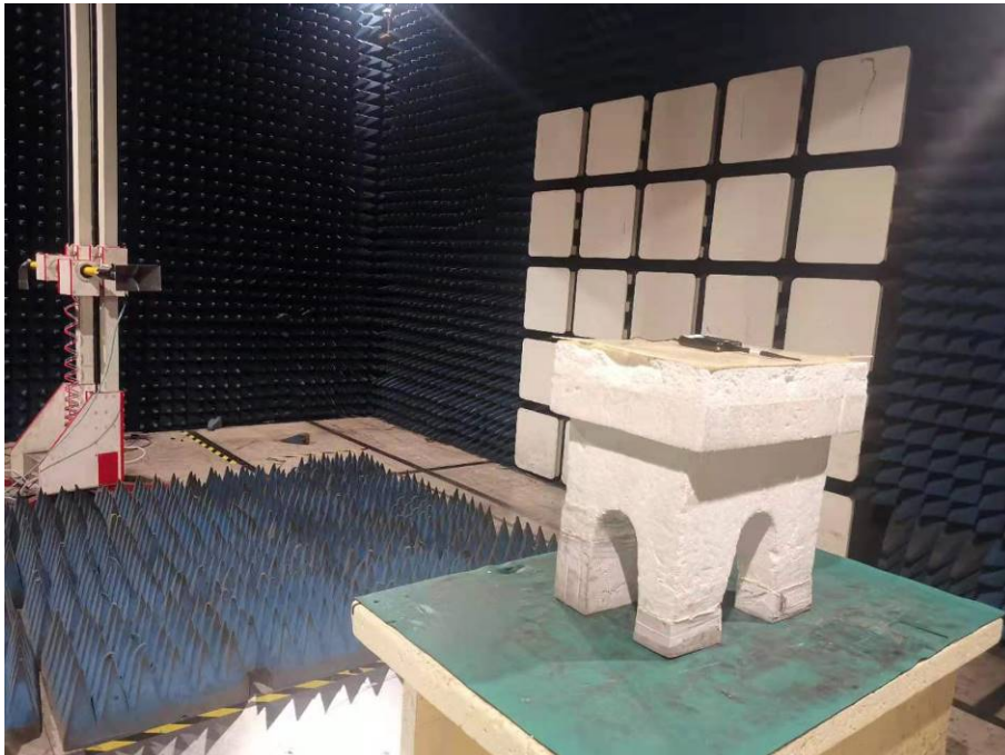
Spurious Emission Test Setup (Above 1GHz)
