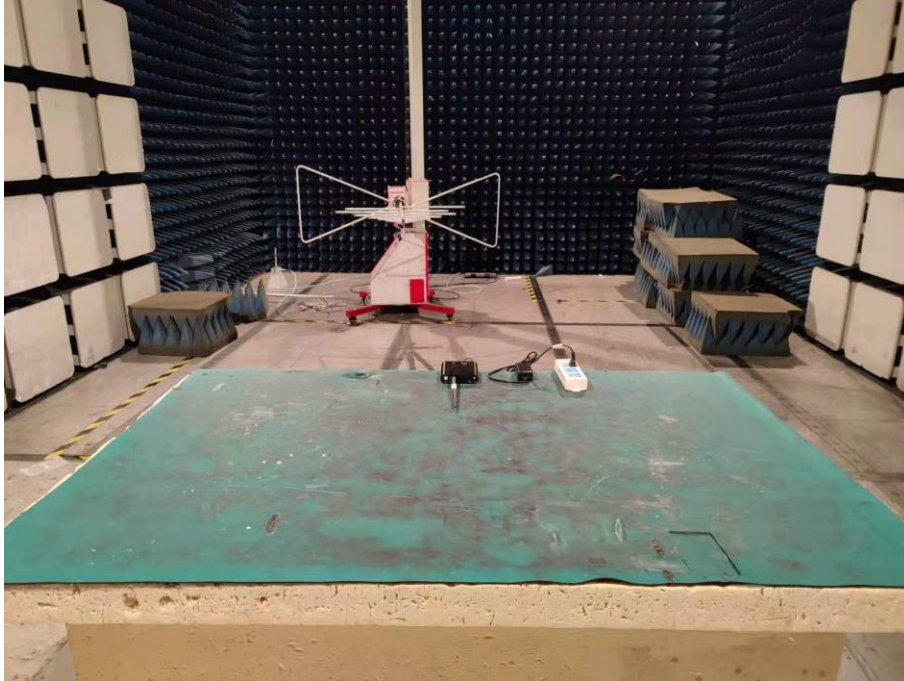
Spurious Emission Test Setup (Above 1GHz)
