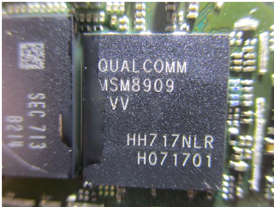
EUT –Main Chip View
