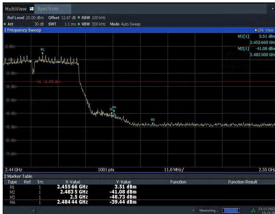
Fig.A.5.8 Band Edges (802.11n-HT40, Ch 9)
