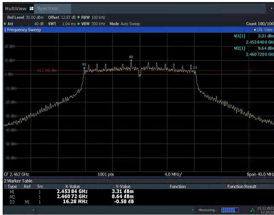
Fig.A.4.6 Occupied 6dB Bandwidth (802.11g, Ch 11)
