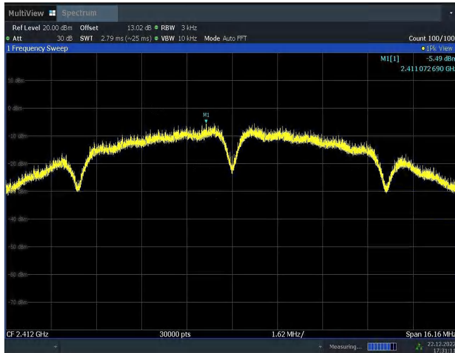
Fig.A.3.1 Power Spectral Density(802.11b,Ch1)
