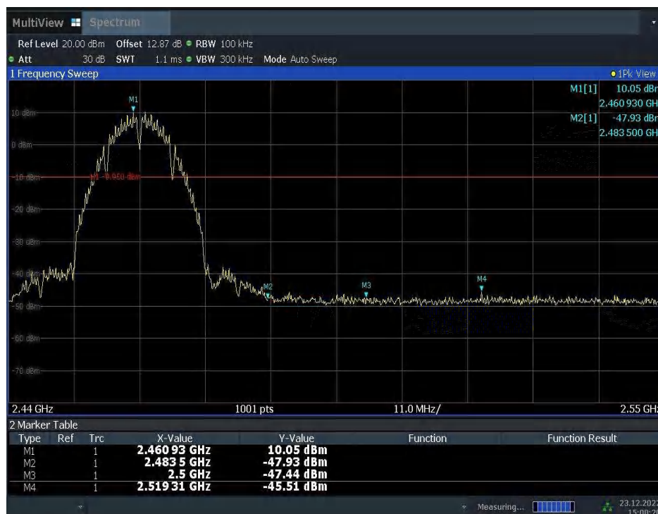
Fig.A.5.2 Band Edges (802.11b, Ch 11)
