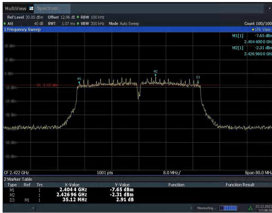
Fig.A.4.10 Occupied 6dB Bandwidth (802.11n-40MHz, Ch 3)
