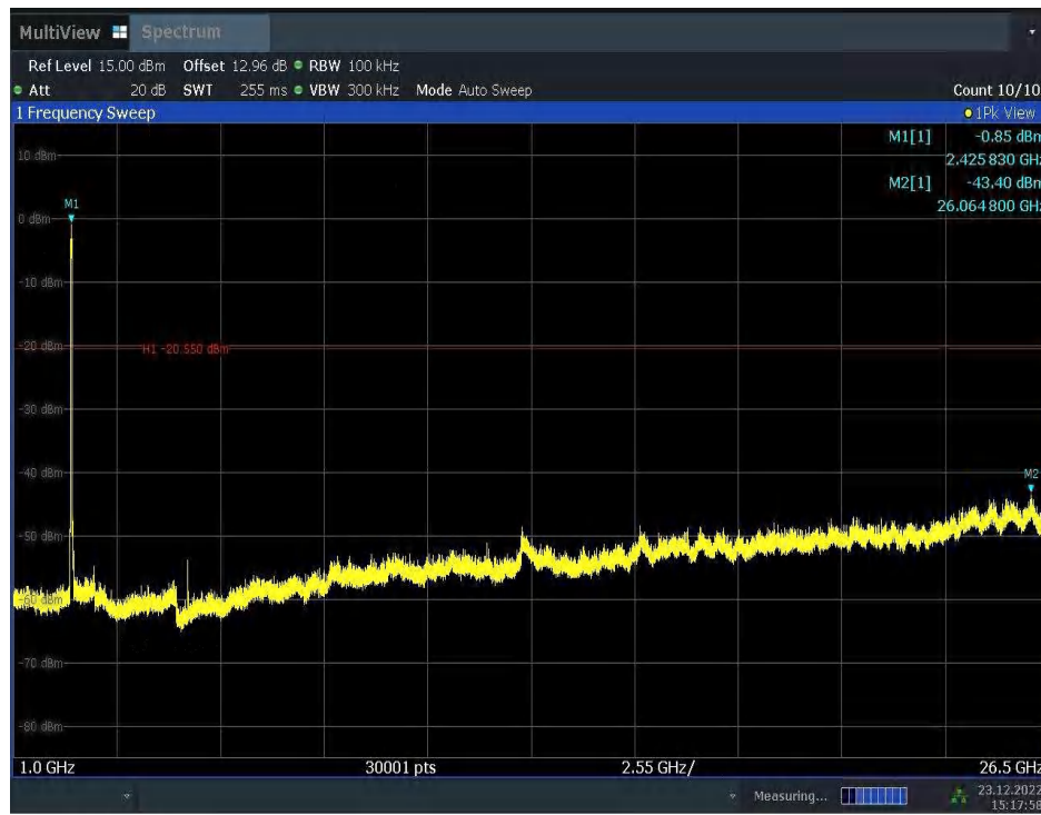
Fig.A.6.1.30 Transmitter Spurious Emission - Conducted (802.11n-HT40, Ch3, 1 GHz-26.5 GHz)
