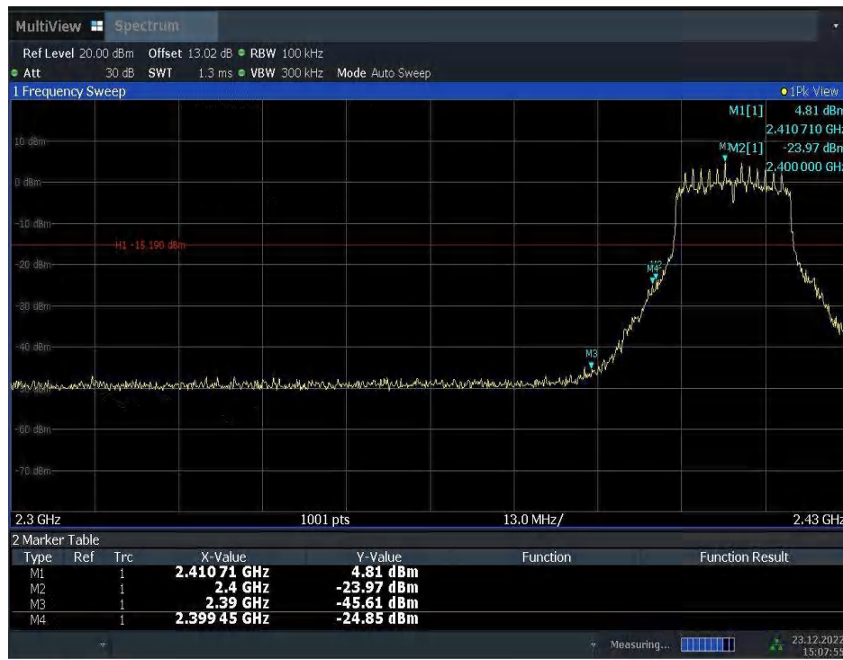
Fig.A.5.5 Band Edges (802.11n-HT20, Ch 1)
