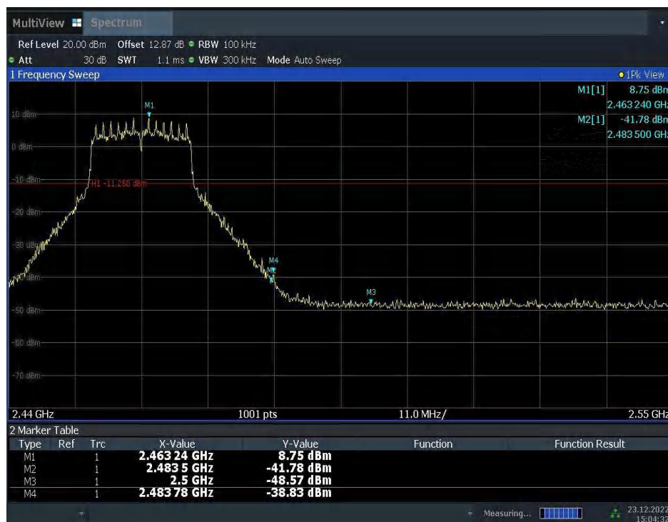
Fig.A.5.4 Band Edges (802.11g, Ch 11)
