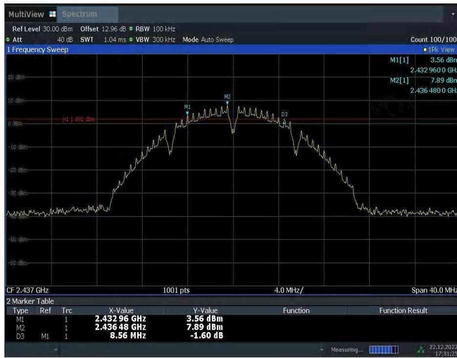
Fig.A.4.2 Occupied 6dB Bandwidth (802.11b, Ch 6)
