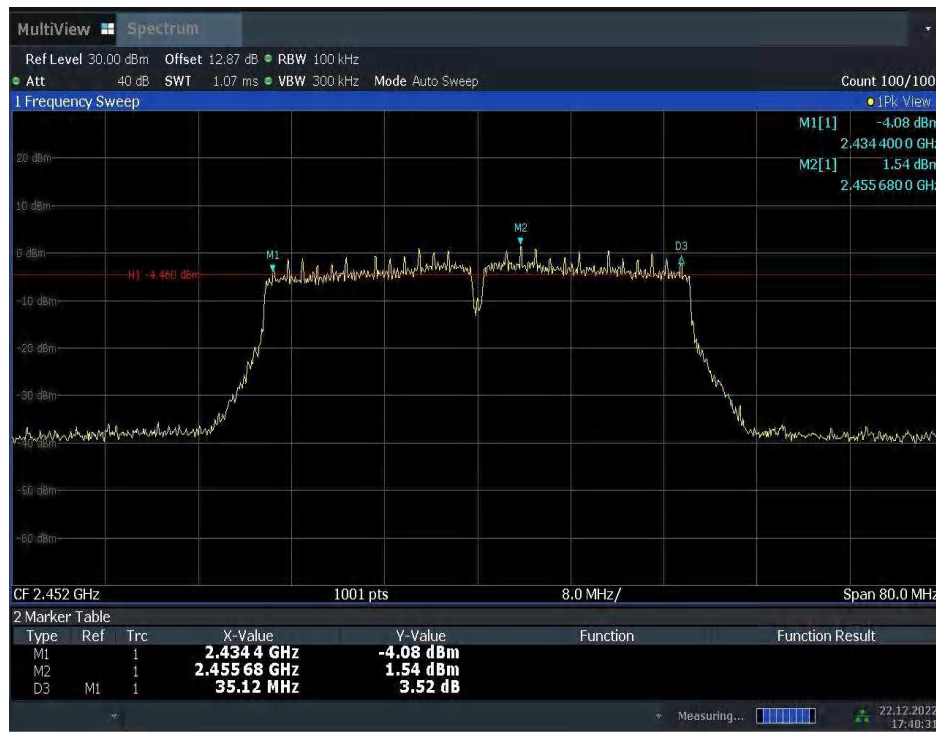
Fig.A.4.12 Occupied 6dB Bandwidth (802.11n-HT40, Ch 9)
