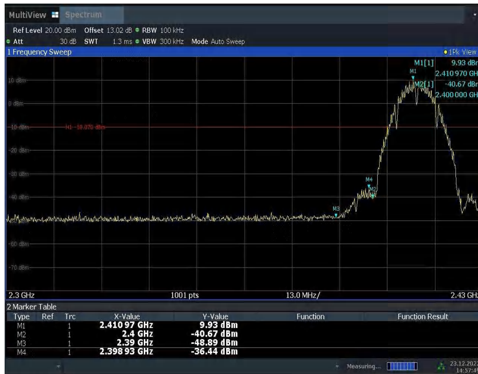
Fig.A.5.1 Band Edges (802.11b, Ch 1)
