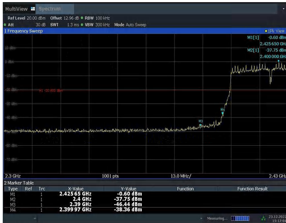
Fig.A.5.7 Band Edges (802.11n-HT40, Ch 3)
