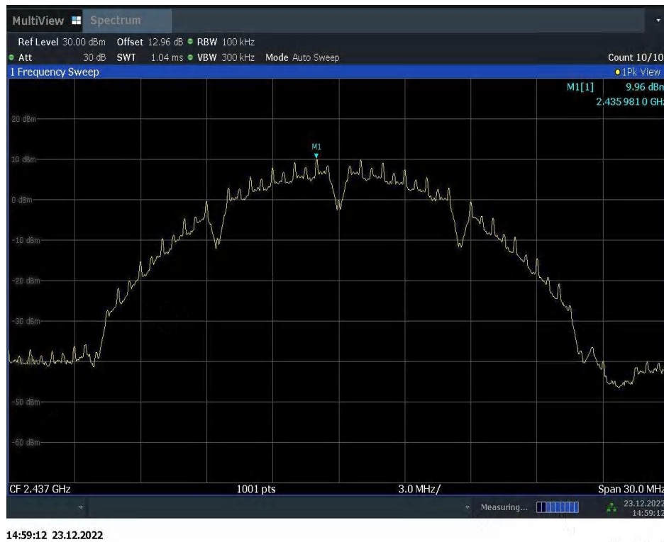
Fig.A.6.1.4 Transmitter Spurious Emission - Conducted (802.11b, Ch6, Center Frequency)
