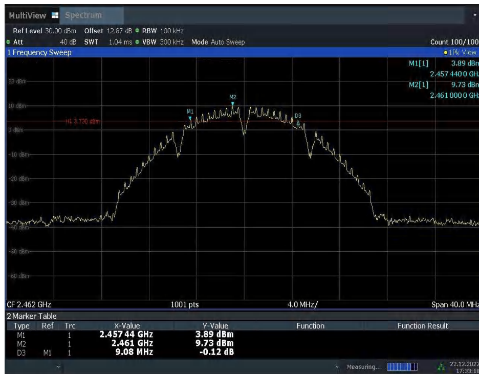
Fig.A.4.3 Occupied 6dB Bandwidth (802.11b, Ch 11)
