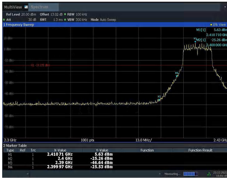
Fig.A.5.3 Band Edges (802.11g, Ch 1)
