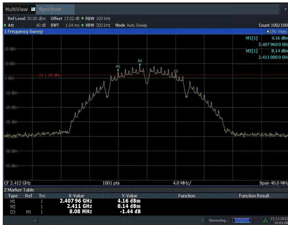
Fig.A.4.1 Occupied 6dB Bandwidth(802.11b,Ch 1)
