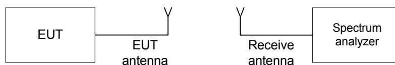
Figure 7.3.1 Occupied bandwidth test setup
