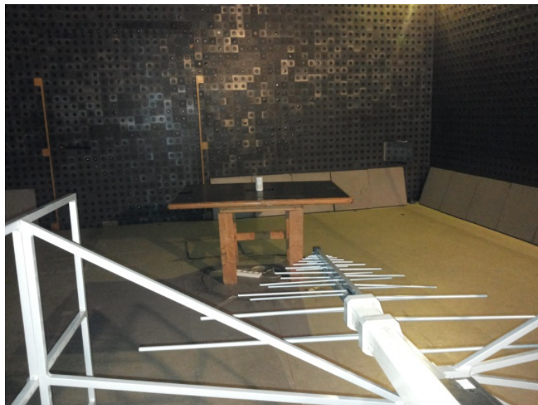
Photograph 8.1.1 Setup for radiated emission measurements
