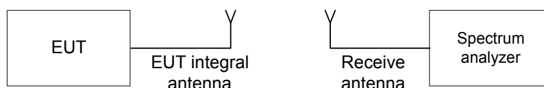
Figure 7.1.1 Setup for transmitter shut down test
