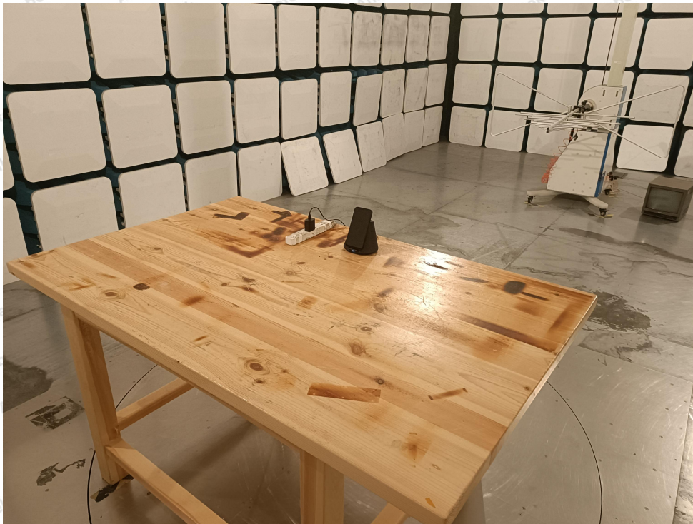
Photo of Radiation Emission Test
