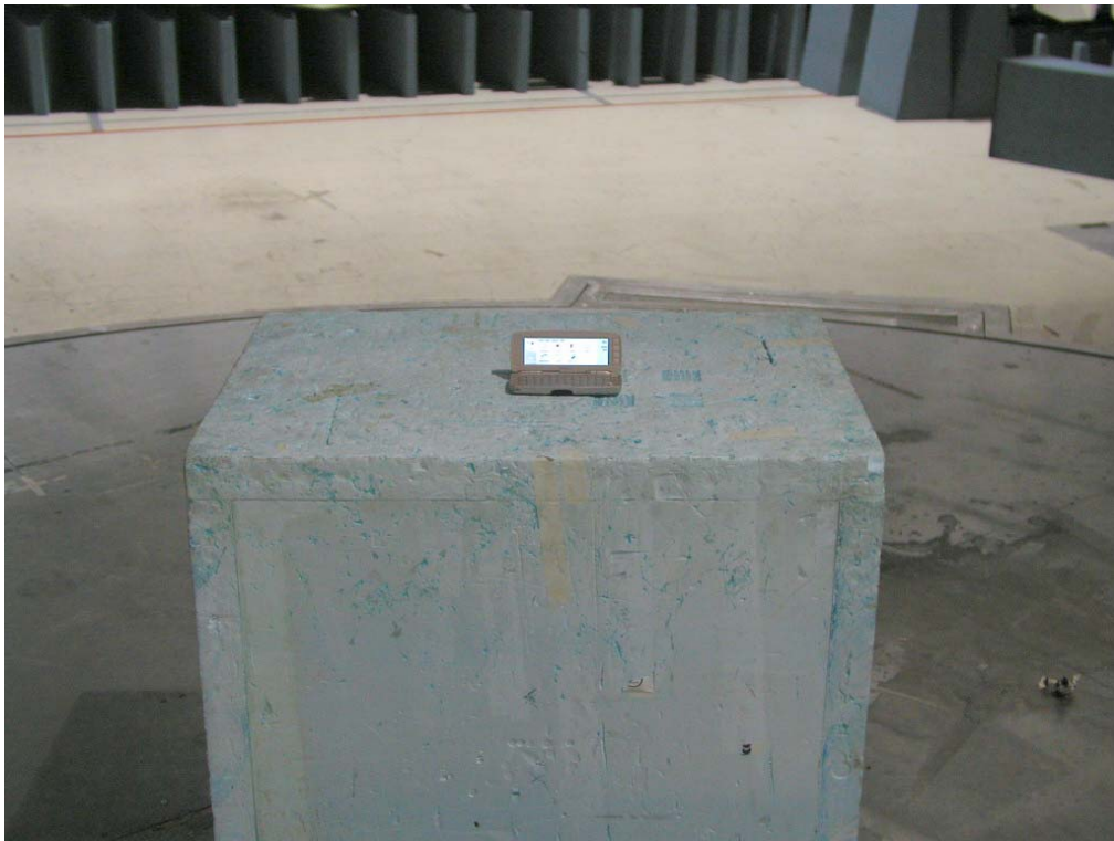
Photograph 1. Radiated RF output power and spurious radiated emissions test setup, flip open
