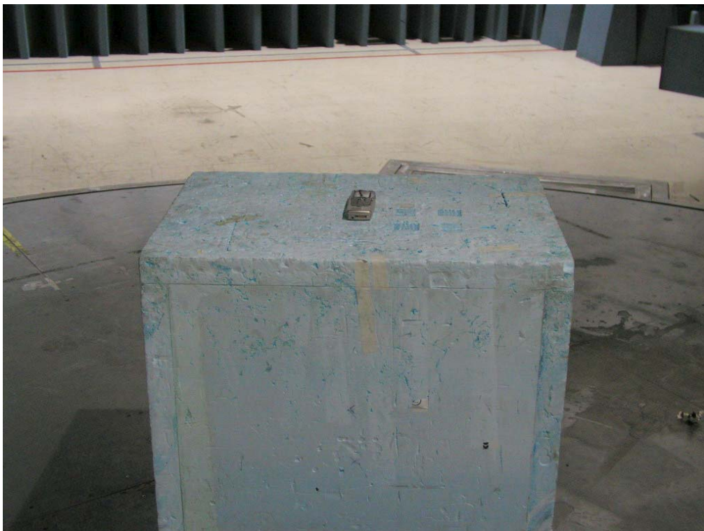
Photograph 2. Radiated RF output power and spurious radiated emissions test setup, flip closed
