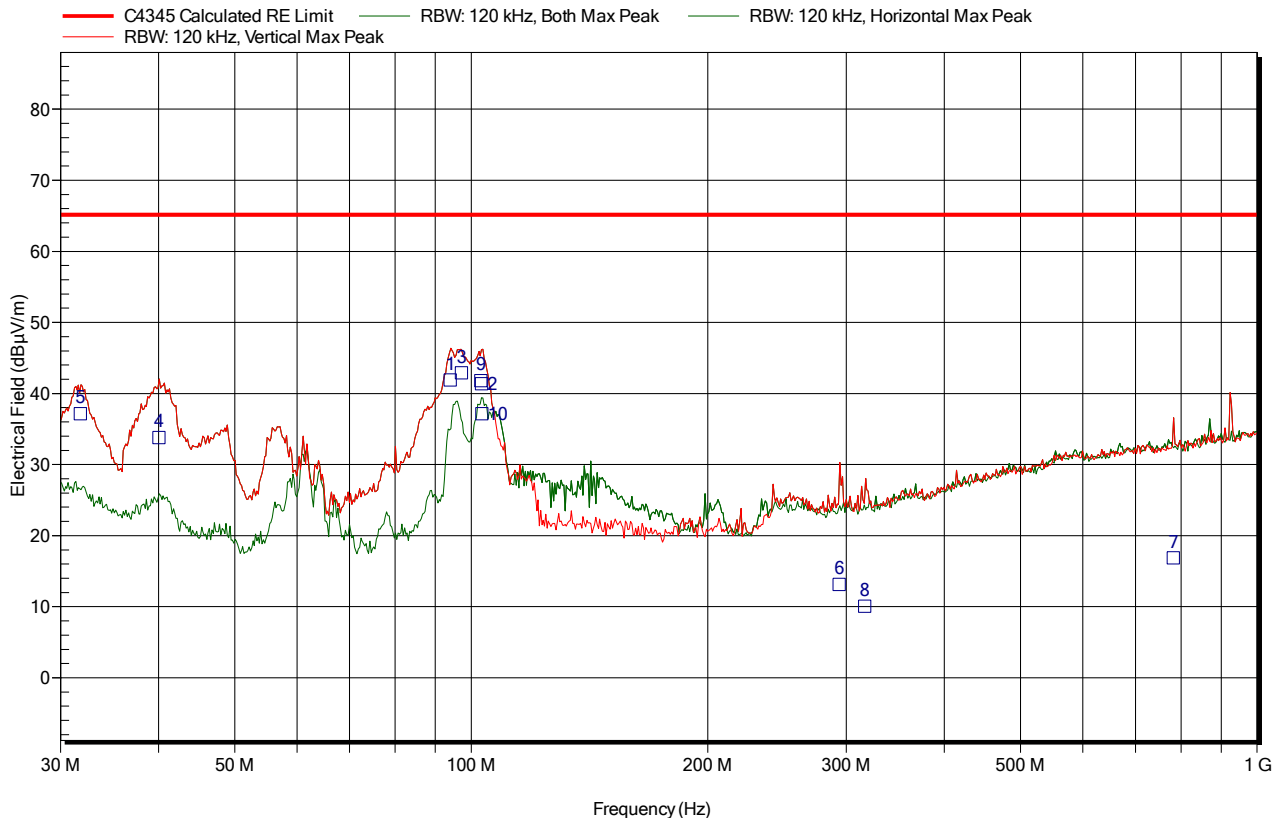
Figure 6: Electric field emissions Plot, 30MHz to 1GHz
