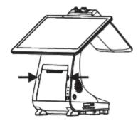
2. Open the built-in printer cover by pressing inward the spring key(that the arrow points to).
