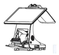
5. Close the printer covers in turn. The "Out of Paper" indicator will light off. The paper is changed successfully.
