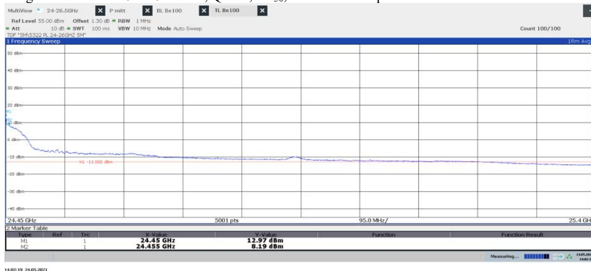
Diagram 2.14d: 24.45 – 25.4 GHz, QPSK, TL 50 , EIRP Vertical polarization
