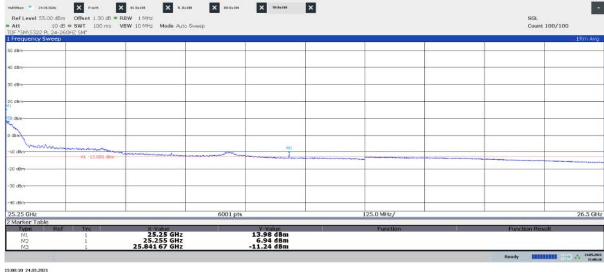
Diagram 2.18c: 25.25 – 26.5 GHz, QPSK, TH 50 , EIRP Horizontal polarization
