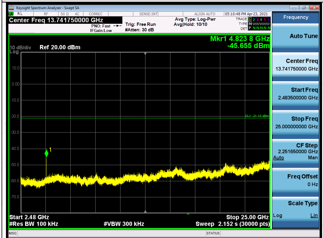
Test_Graph_802.11n20_ANT1_2412_MCS0_Higher Band Emissions
