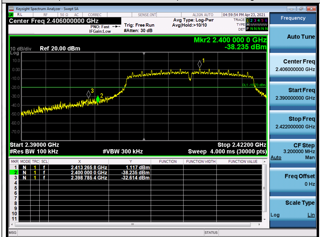
Test_Graph_802.11g_ANT1_2412_6Mbps_Lower Band Edge Emissions
