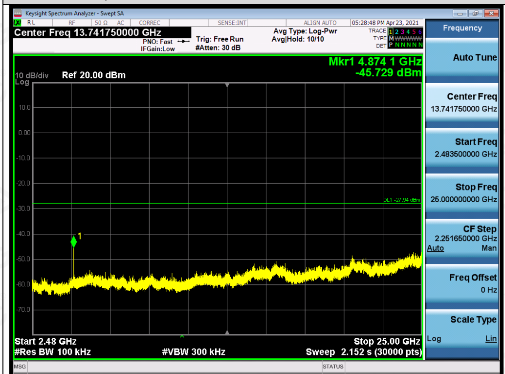
Test_Graph_802.11n40_ANT1_2437_MCS0_Higher Band Emissions
