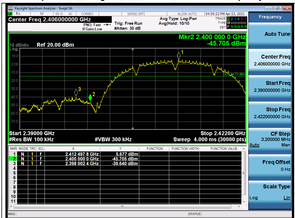
Test_Graph_802.11b_ANT1_2412_1Mbps_Lower Band Edge Emissions
