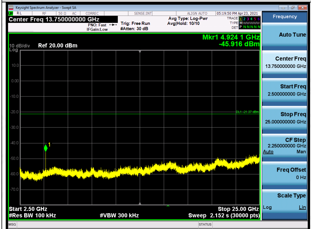
Test_Graph_802.11n20_ANT1_2462_MCS0_Higher Band Emissions
