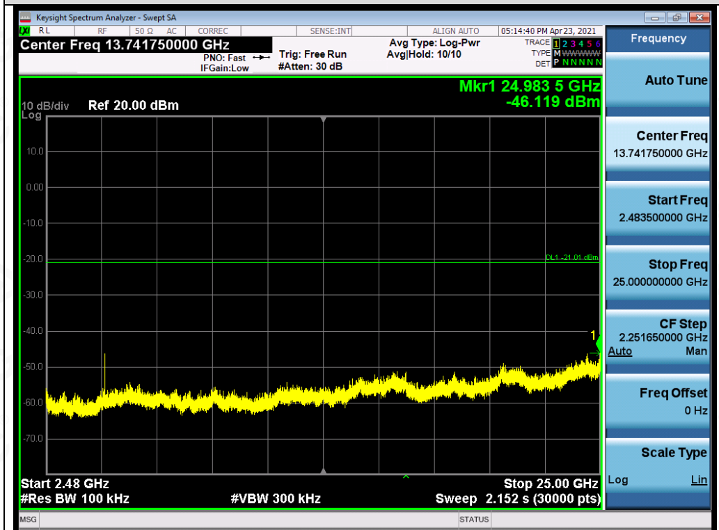
Test_Graph_802.11n20_ANT1_2437_MCS0_Higher Band Emissions
