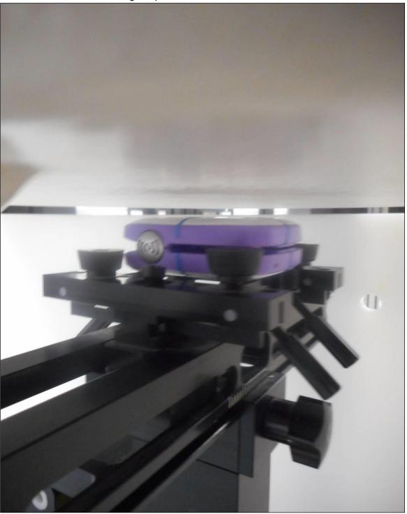
PHT/007: Back of EUT facing the phantom at 7mm
