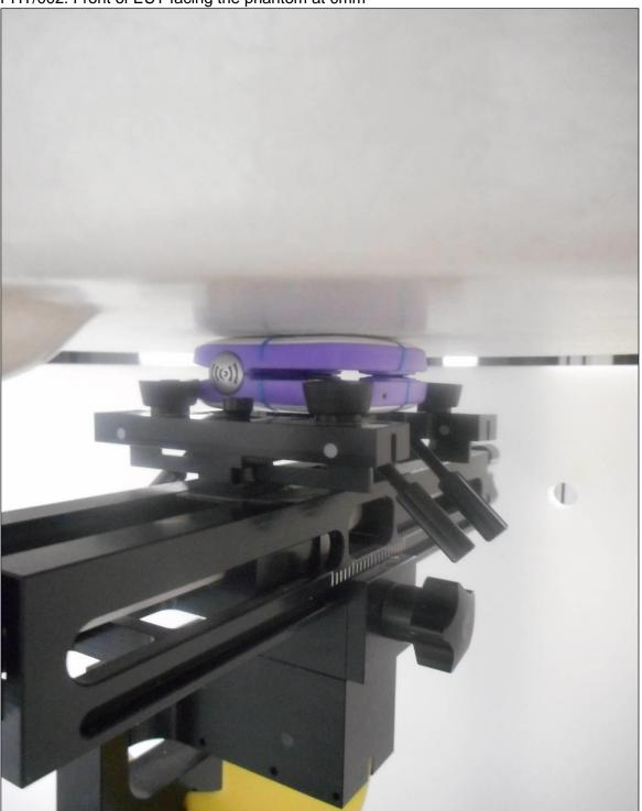
PHT/003: Back of EUT facing the phantom at 0mm
