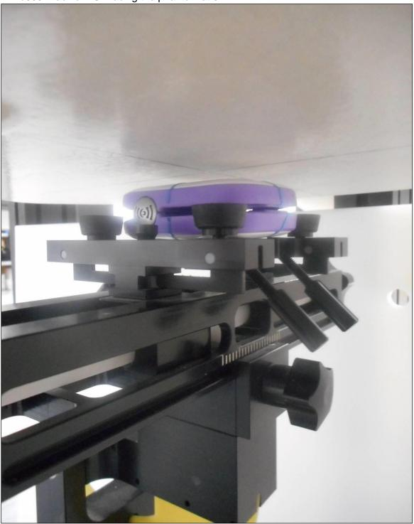
PHT/006: Front of EUT facing the phantom at 7mm
