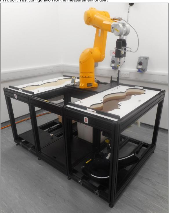
PHT/002: Front of EUT facing the phantom at 0mm
