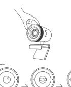
Tripod screw hole is located at the Manually adjust the webcam tilt up/down or bottom of the clip mount for tripod swivel right/left to the best shooting angle. mounting.
