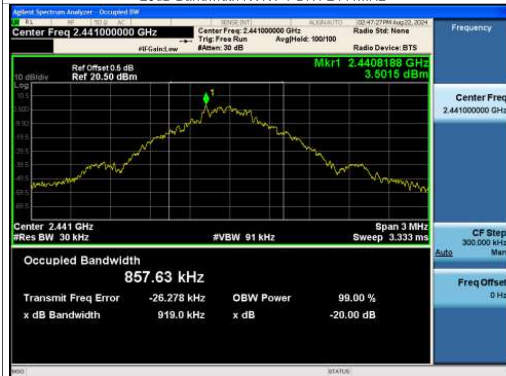
-20dB Bandwidth NVNT 1-DH1 2441MHz
