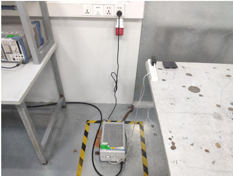
FCC ID: : 2AWOQ-003001C590 Photo of Power Line Conducted Emission Test
