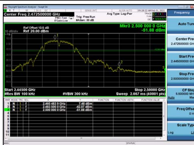
,Plot 2,Band Edge-802.11b,2462MHz
