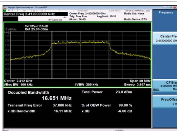
6dB Bandwidth-802.11g,2462MHz
