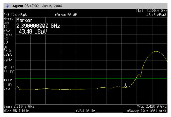
Detector mode: Peak Polarity: Horizontal
