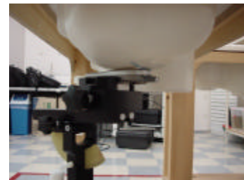
Fig. 15. Head SAR Test Setup
