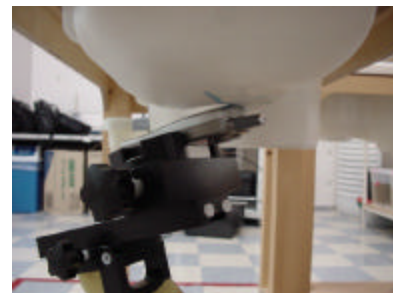
Fig. 17. Head SAR Test Setup
