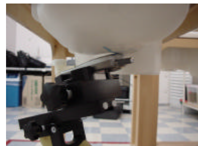
Fig. 19. Head SAR Test Setup
