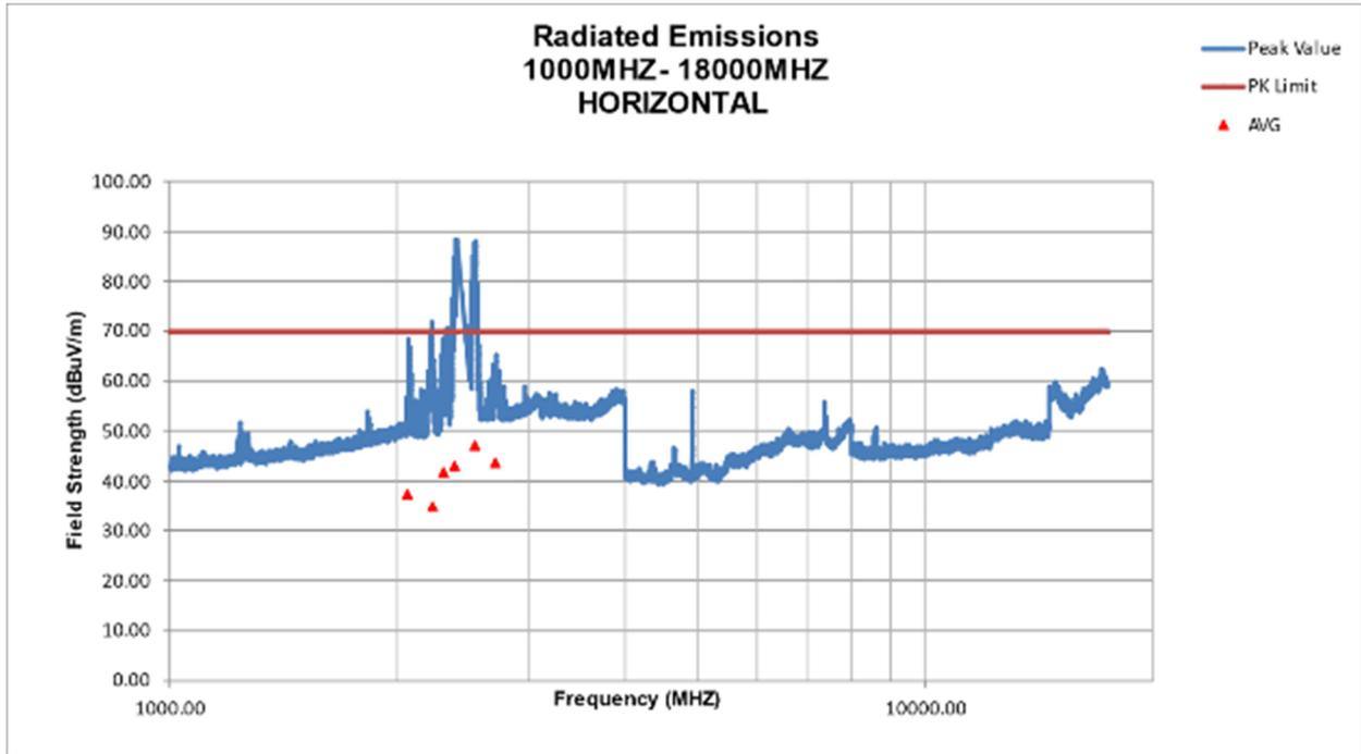
Figure 6. Radiated Emissions Above 1 GHz Horizontal
