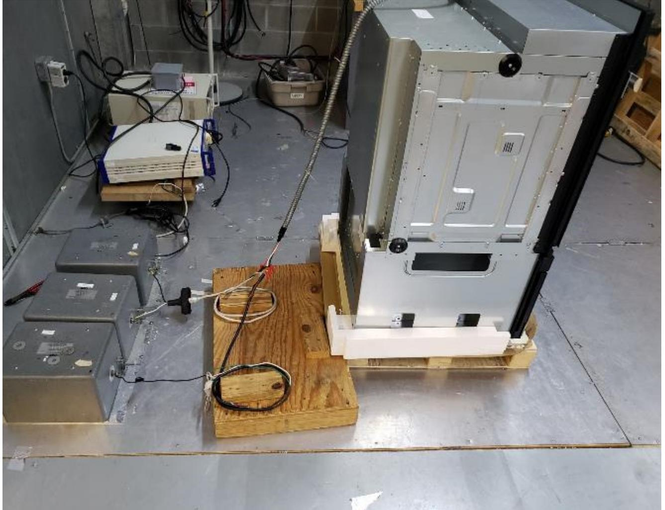
**Figure 8. Photograph of Conducted Emissions Test Configuration**
