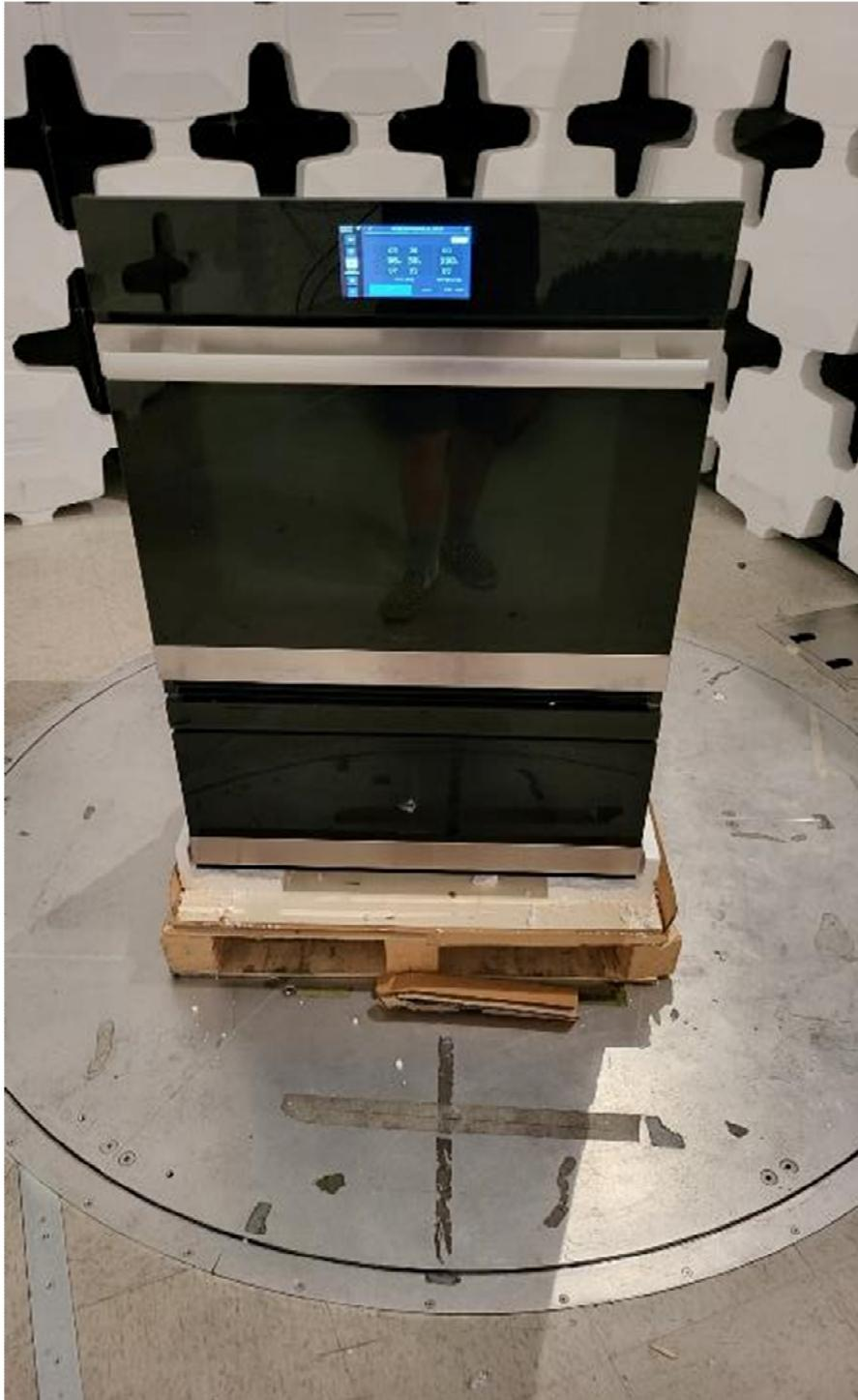
**Figure 9. Photograph of Radiated Emissions Test Configuration, Close-Up**
