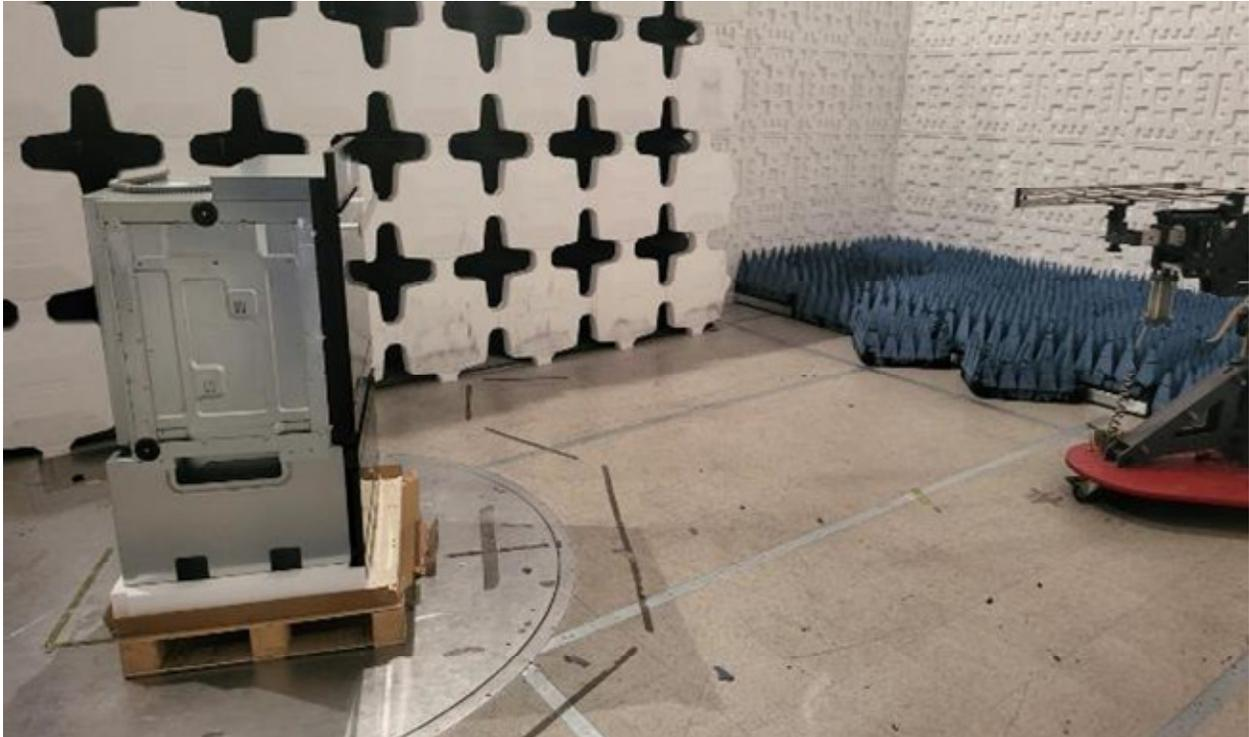
**Figure 11. Photograph of Radiated Emissions Test Configuration, 200 - 1000 MHz**
