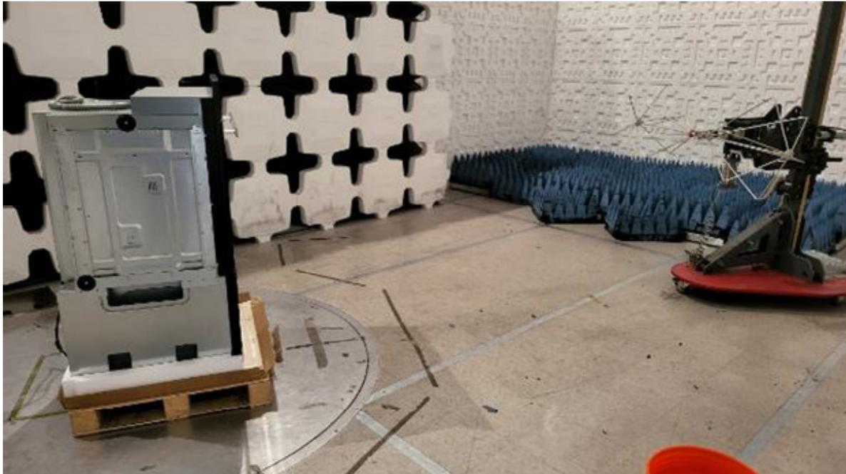
**Figure 10. Photograph of Radiated Emissions Test Configuration, 30 - 200 MHz**
