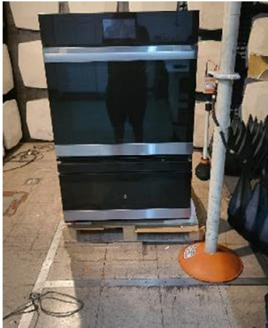
**Figure 16. Radiation Leakage Setup**
