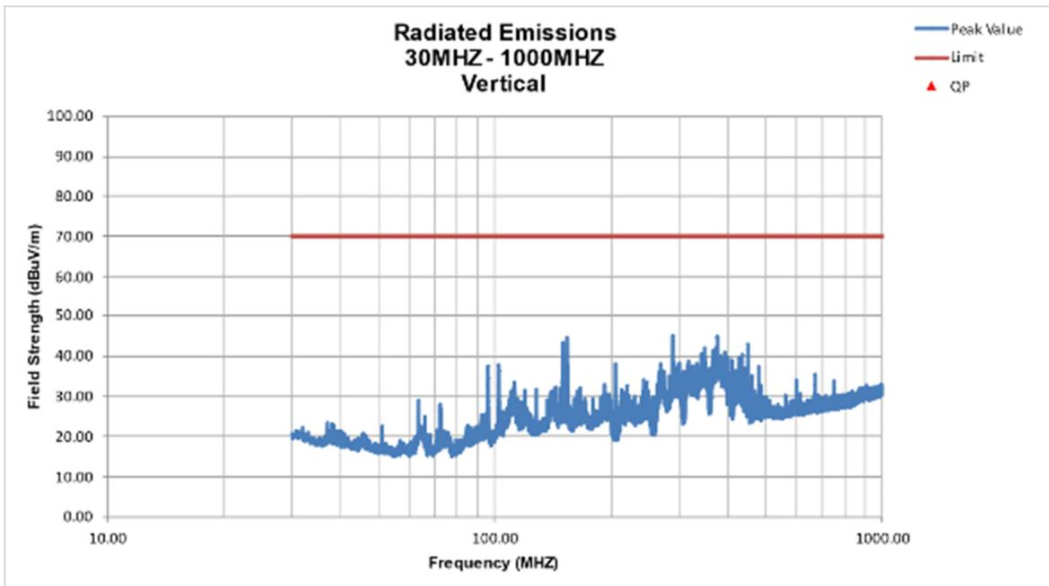
Figure 5. Radiated Emissions Below 30-1000 MHz Vertical
