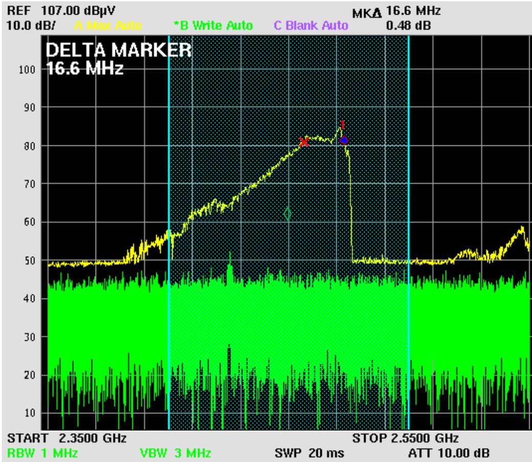
Figure 13. Frequency Variation at Nominal Voltage
