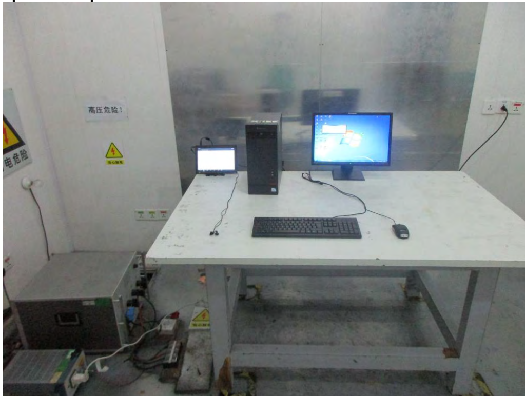
Photograph 2: Set-up for Radiated Emission of below 1GHz
