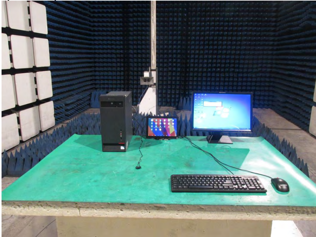
Photograph 3: Set-up for Radiated Emission of 1 - 18GHz
