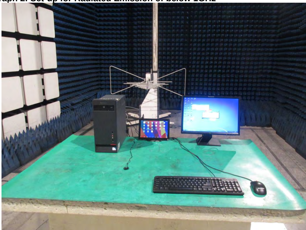
Photograph 2: Set-up for Radiated Emission of below 1GHz
