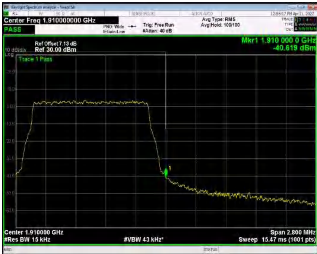
Band2 QPSK BW=10MHz Channel=18650 RB Size=50 Position=#0
