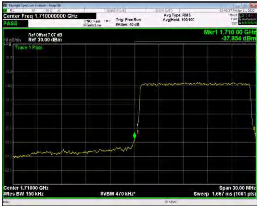
Band4 QPSK BW=15MHz Channel=20325 RB Size=75 Position=#0
