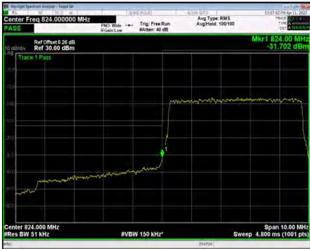
Band5 QPSK BW=5MHz Channel=20625 RB Size=25 Position=#0
