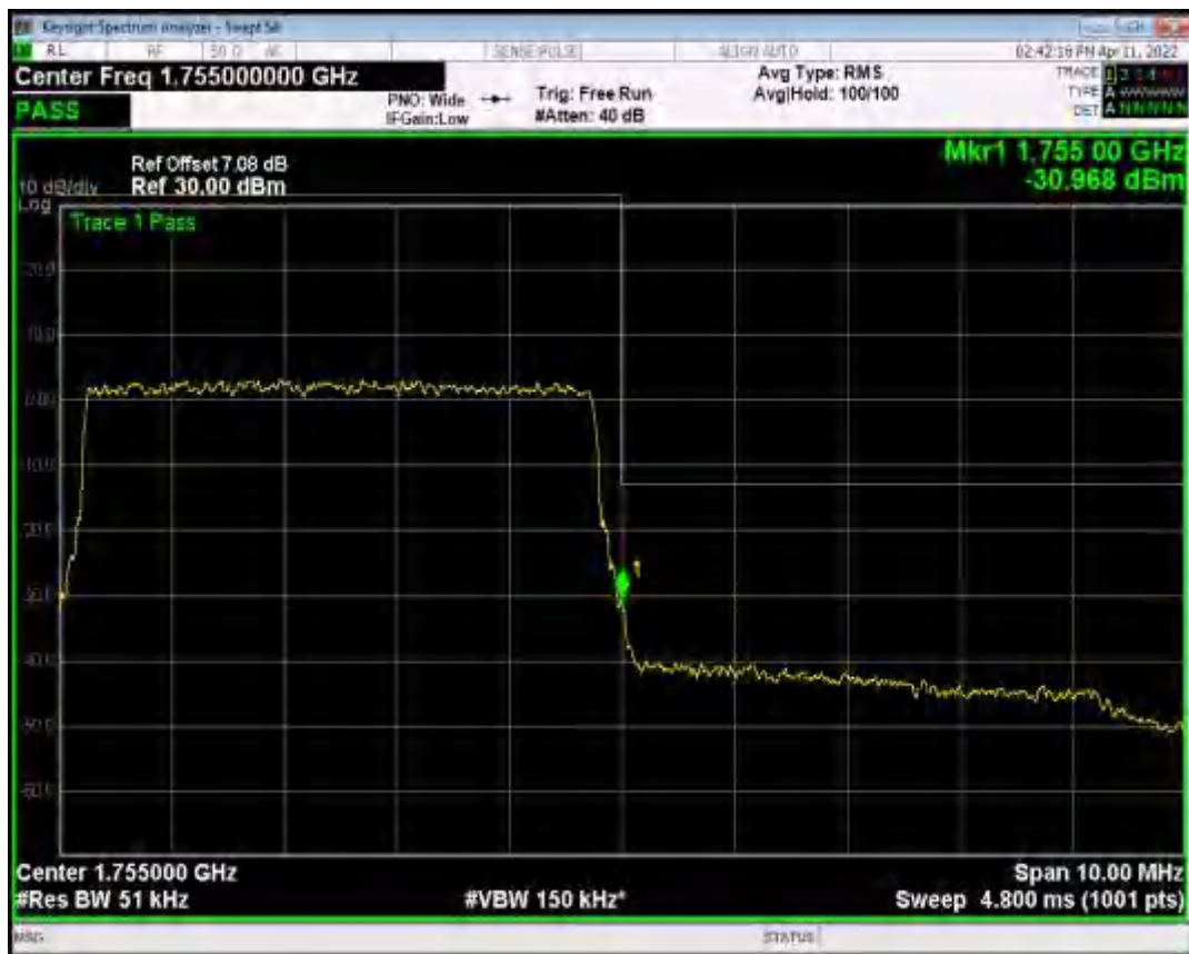
Band5 QAM16 BW=1.4MHz Channel=20407 RB Size=6 Position=#0
