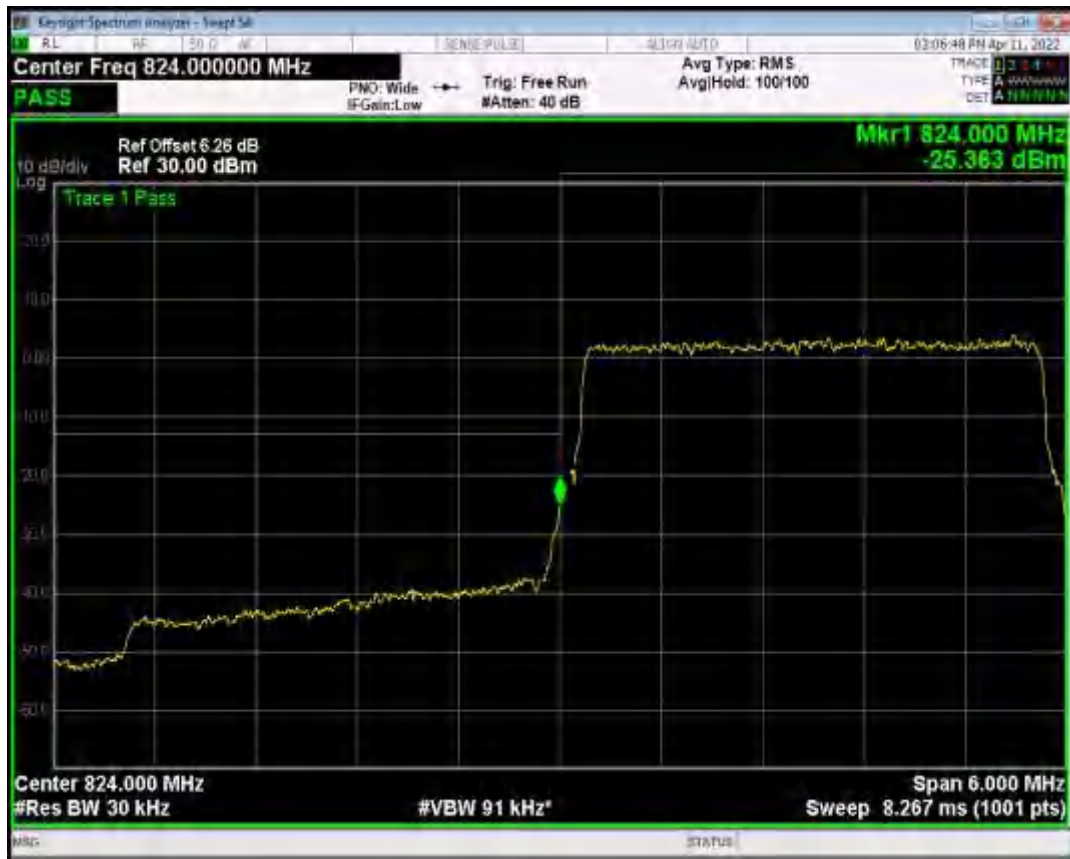
Band5 QPSK BW=3MHz Channel=20635 RB Size=15 Position=#0
