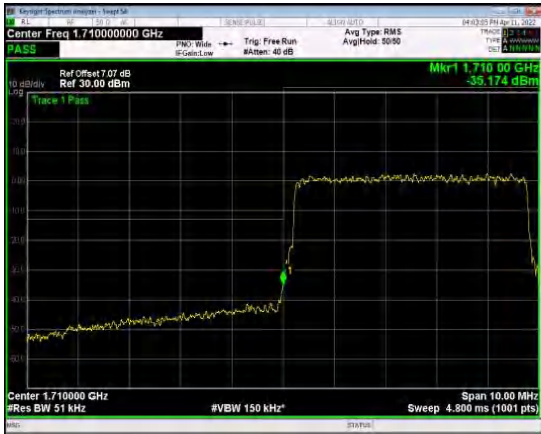
Band66 QAM16 BW=5MHz Channel=132647 RB Size=25 Position=#0
