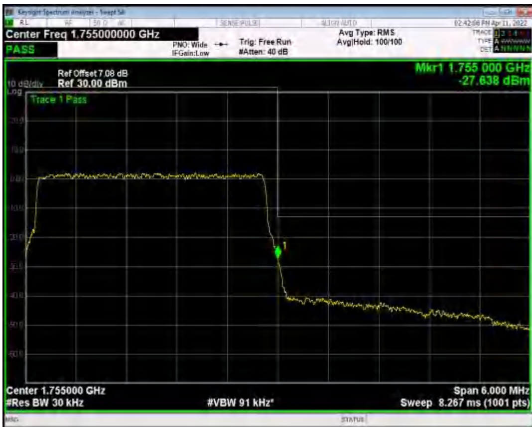
Band4 QAM16 BW=5MHz Channel=19975 RB Size=25 Position=#0
