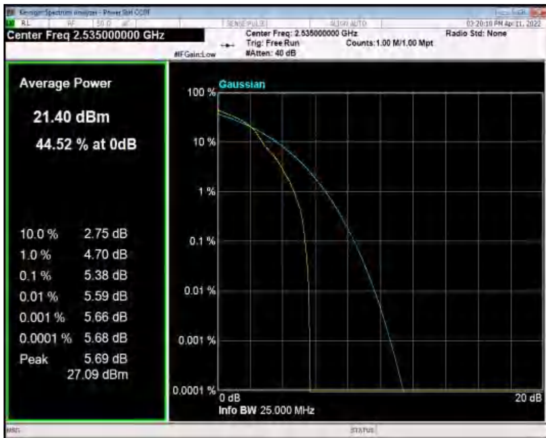
Band7 QAM16 BW=15MHz Channel=21100 RB Size=1 Position=#0
