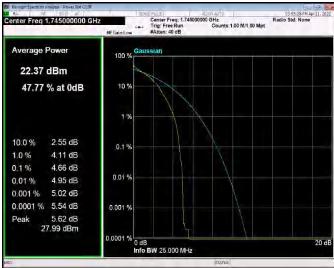
Band66 QPSK BW=3MHz Channel=132322 RB Size=1 Position=#0
