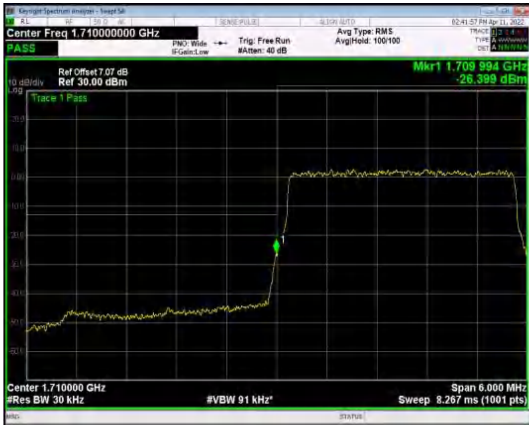
Band4 QPSK BW=3MHz Channel=20385 RB Size=15 Position=#0
