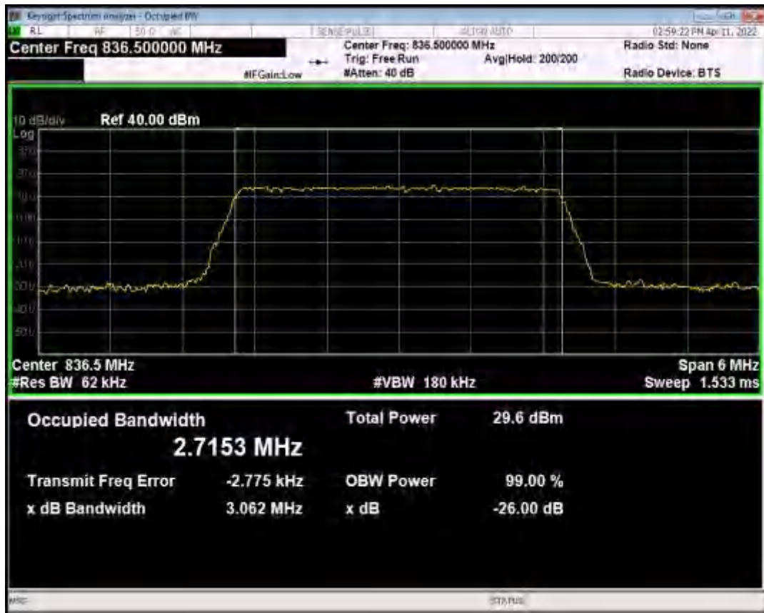
Band5 QPSK BW=5MHz Channel=20525 RB Size=25 Position=#0
