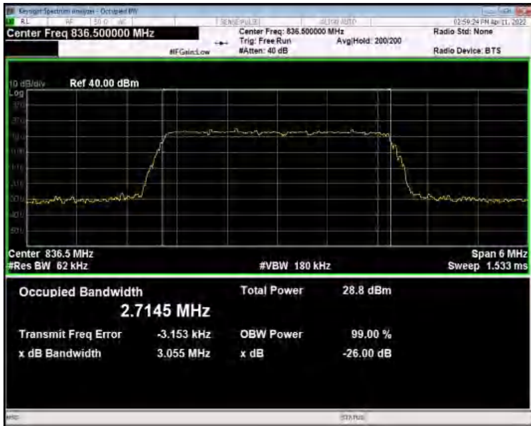
Band5 QAM16 BW=5MHz Channel=20525 RB Size=25 Position=#0
