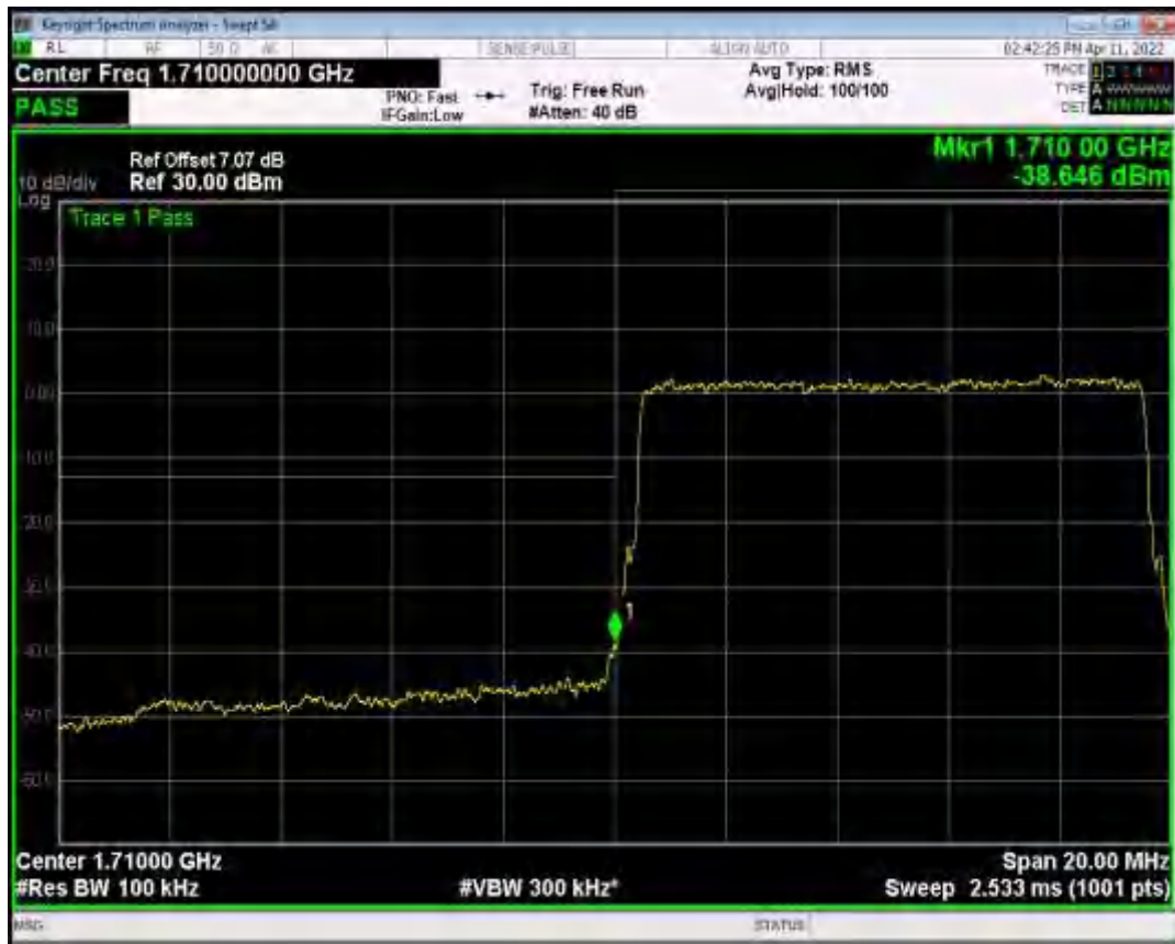
Band4 QPSK BW=10MHz Channel=20350 RB Size=50 Position=#0
