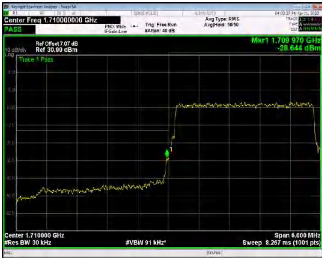
Band66 QPSK BW=3MHz Channel=132657 RB Size=15 Position=#0
