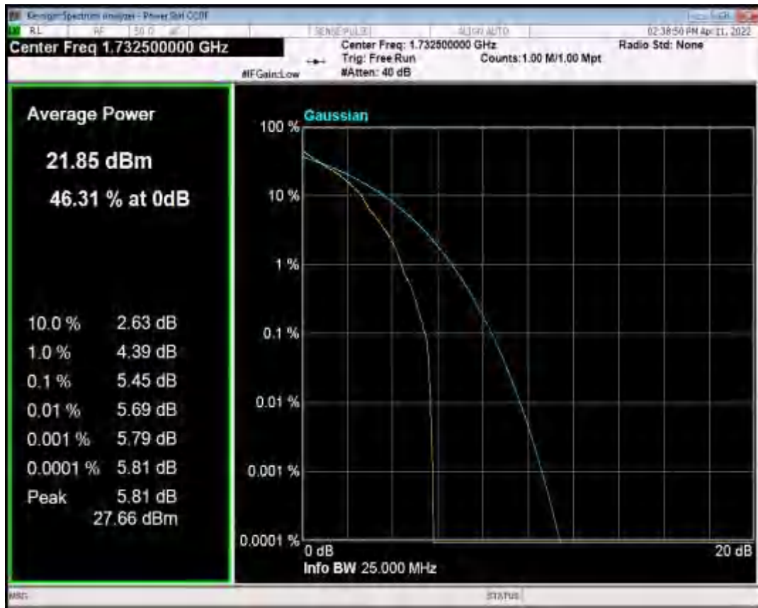
Band5 QAM16 BW=1.4MHz Channel=20525 RB Size=1 Position=#0
