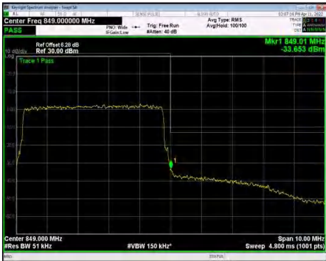
Band5 QPSK BW=1.4MHz Channel=20407 RB Size=6 Position=#0
