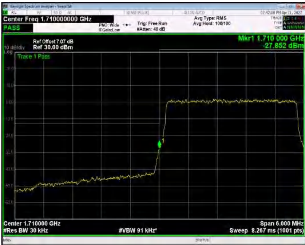
Band4 QAM16 BW=3MHz Channel=20385 RB Size=15 Position=#0
