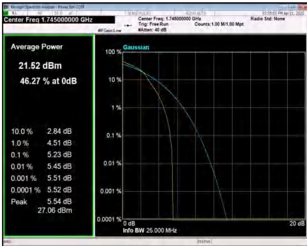
Band66 QAM16 BW=10MHz Channel=132322 RB Size=1 Position=#0
