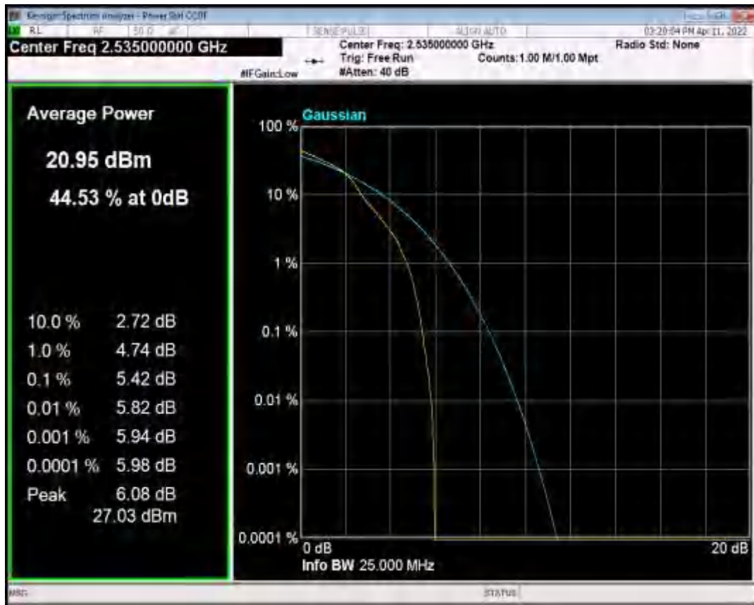
Band7 QPSK BW=10MHz Channel=21100 RB Size=1 Position=#0
