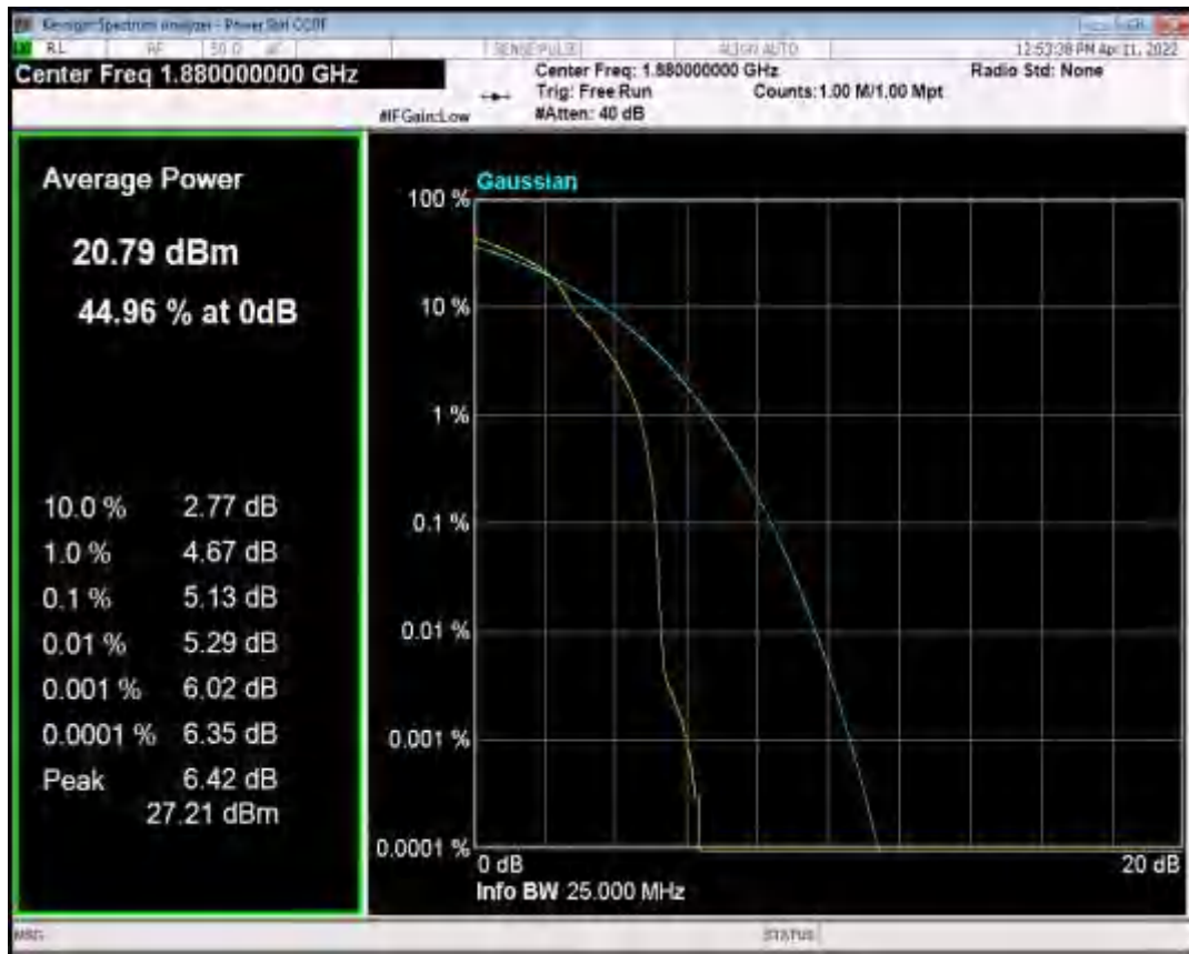
Band2 QAM16 BW=3MHz Channel=18900 RB Size=1 Position=#0
