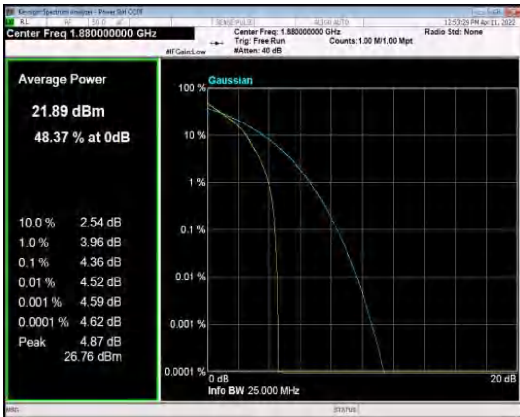
Band2 QPSK BW=20MHz Channel=18900 RB Size=1 Position=#0
