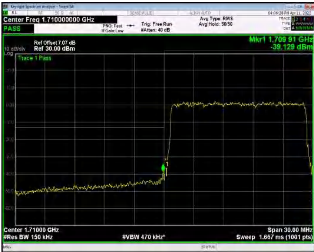
Band66 QAM16 BW=15MHz Channel=132597 RB Size=75 Position=#0
