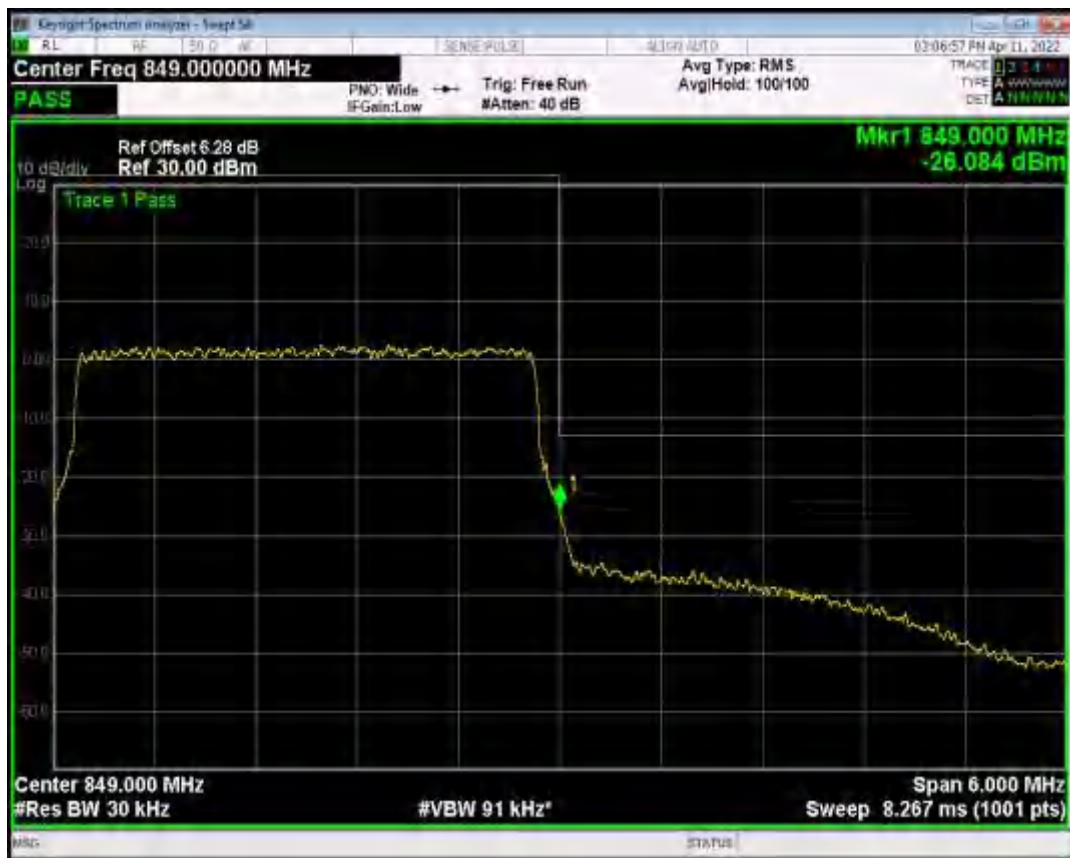
Band5 QAM16 BW=5MHz Channel=20425 RB Size=25 Position=#0
