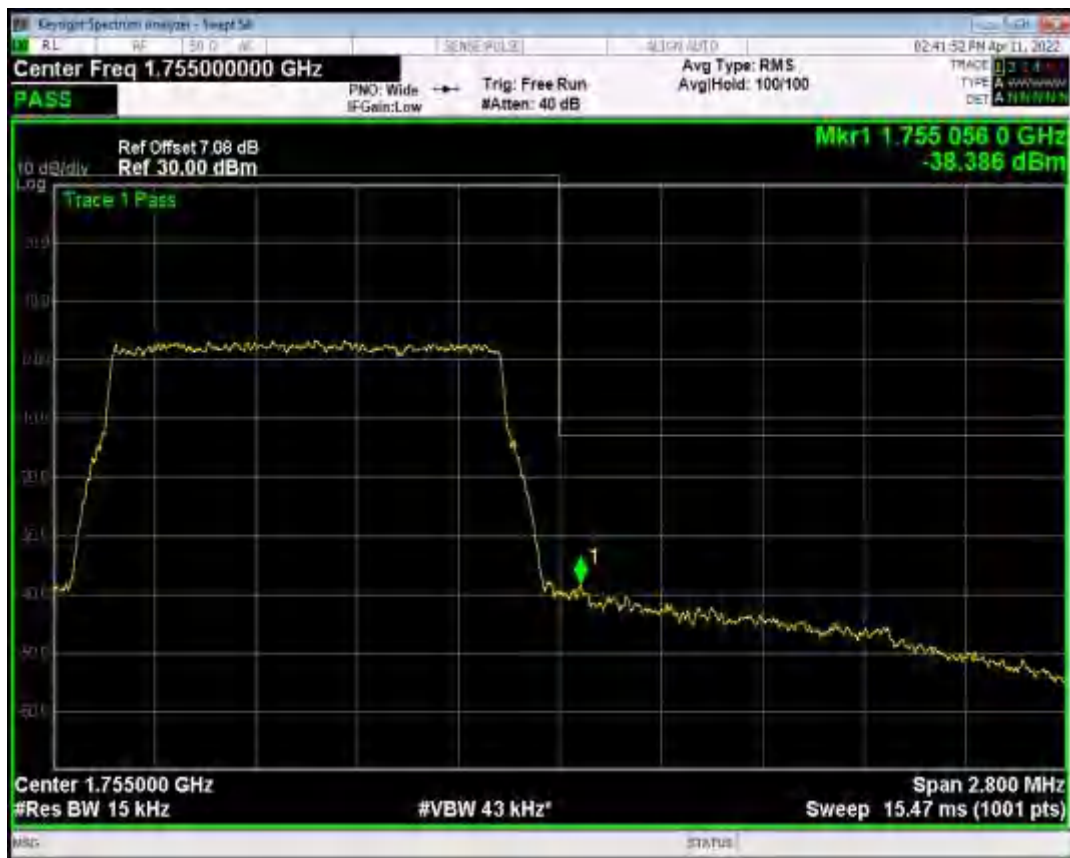
Band4 QAM16 BW=10MHz Channel=20000 RB Size=50 Position=#0
