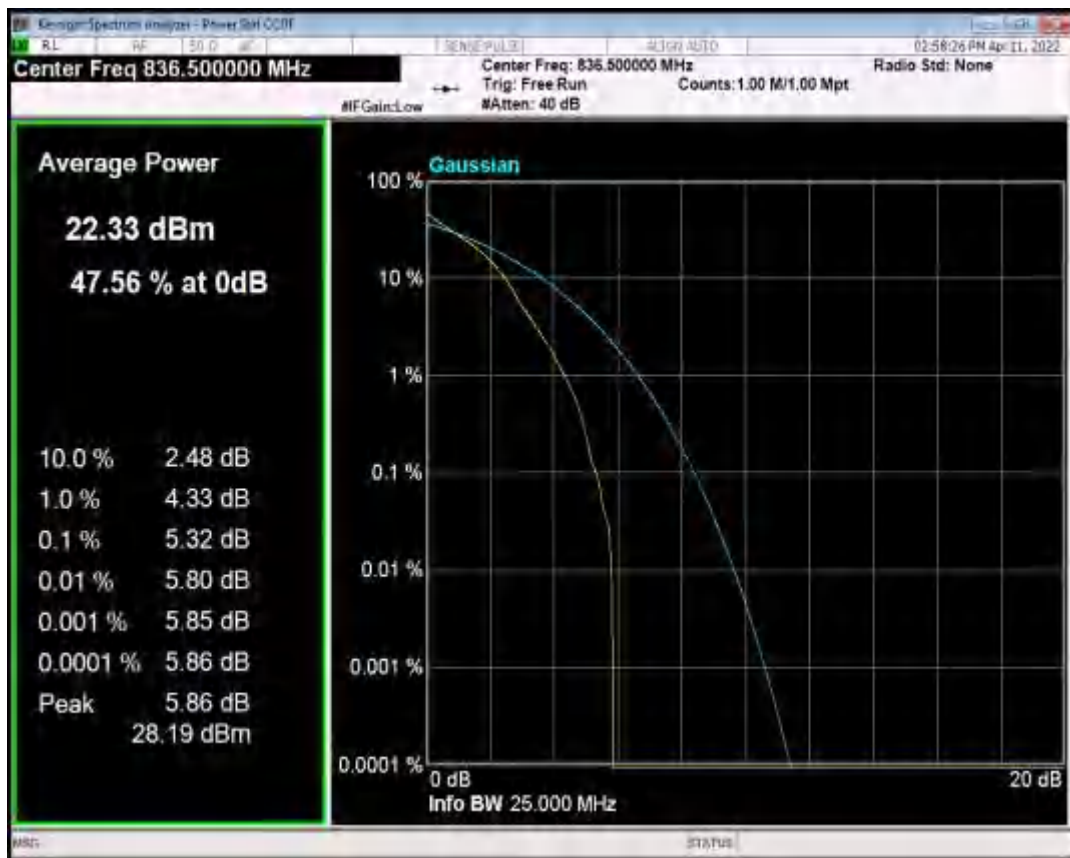
Band5 QPSK BW=10MHz Channel=20525 RB Size=1 Position=#0
