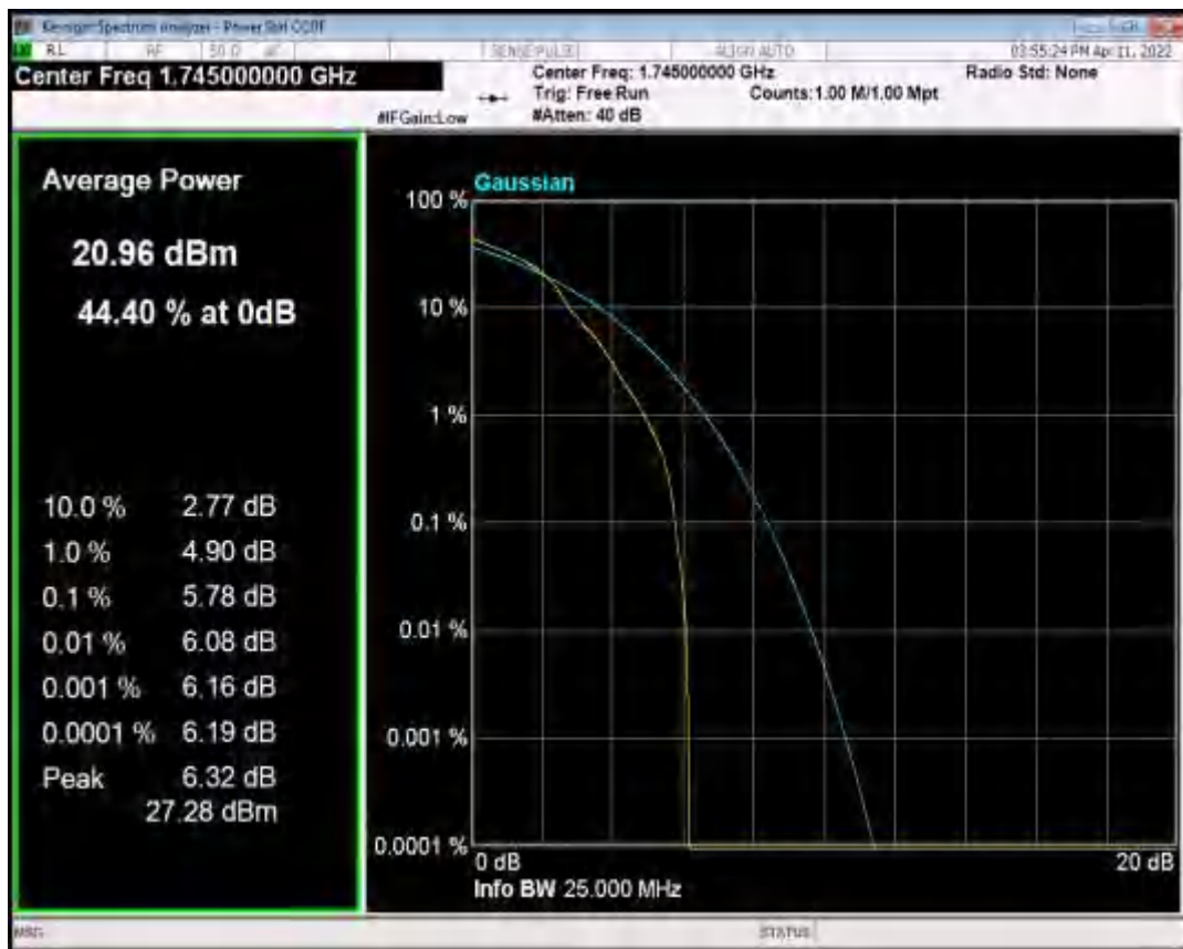
Band66 QAM16 BW=20MHz Channel=132322 RB Size=1 Position=#0
