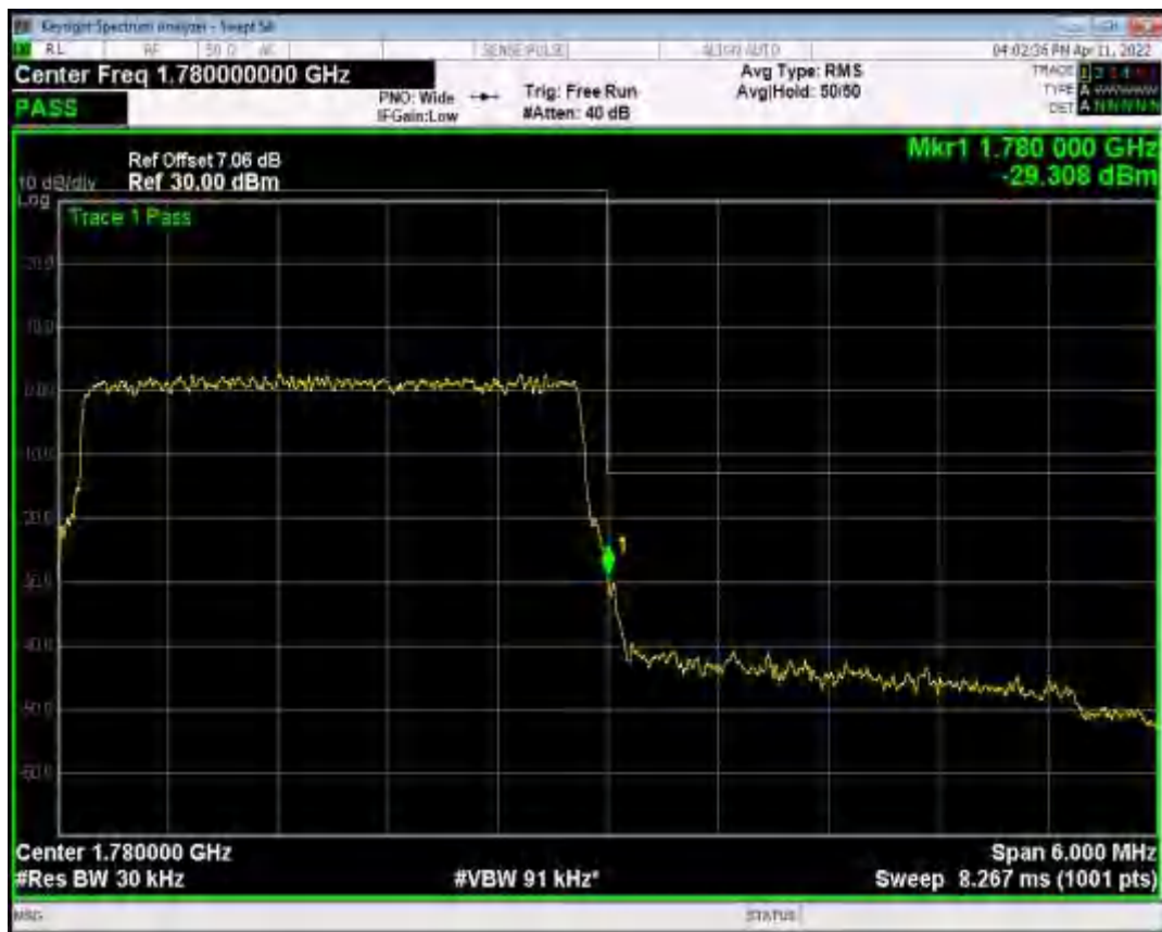
Band66 QAM16 BW=5MHz Channel=131997 RB Size=25 Position=#0
