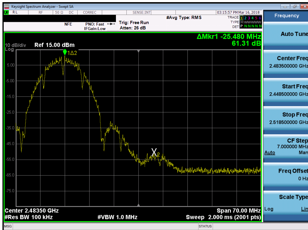
Plot 7-38. Band Edge Plot (802.11b – Ch. 11)
