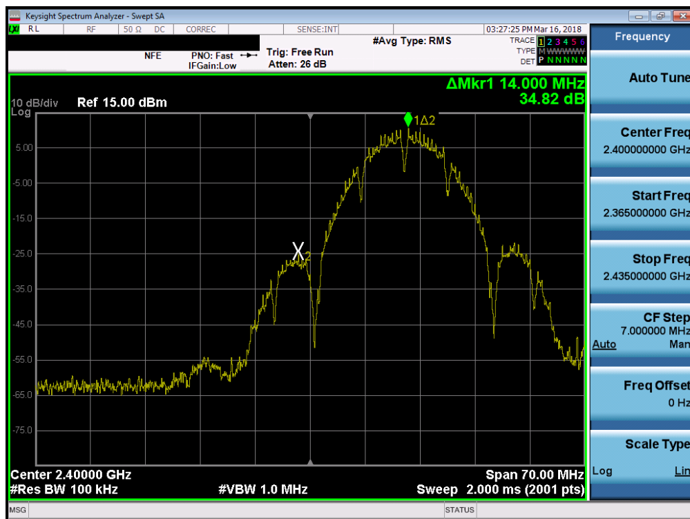
Plot 7-43. Band Edge Plot (802.11b – Ch. 1)
