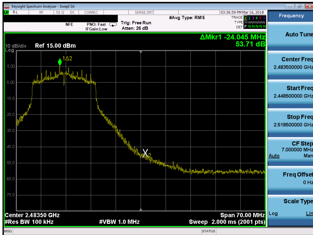
Plot 7-48. Band Edge Plot (802.11n (2.4GHz) – Ch. 11)
