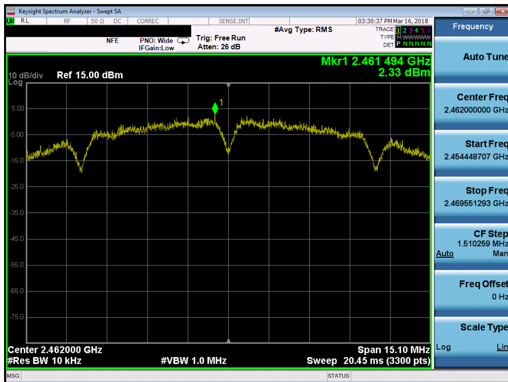
Plot 7-30. Power Spectral Density Plot (802.11b – Ch. 11)
