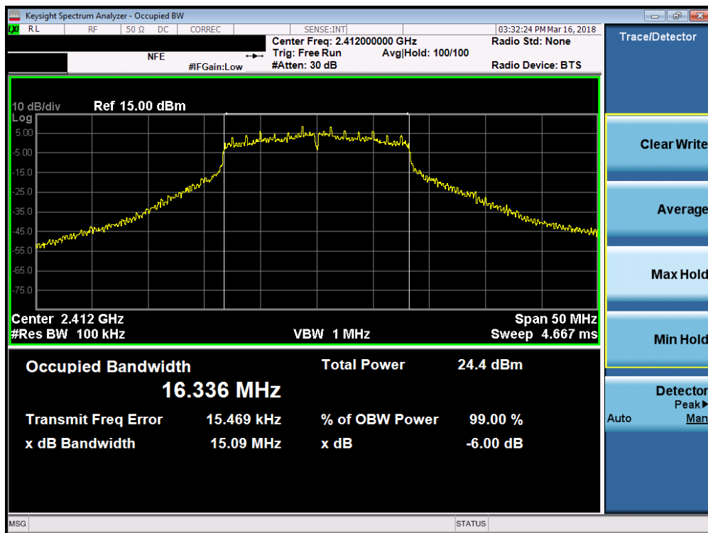
Plot 7-13. 6dB Bandwidth Plot (802.11g – Ch. 1)
