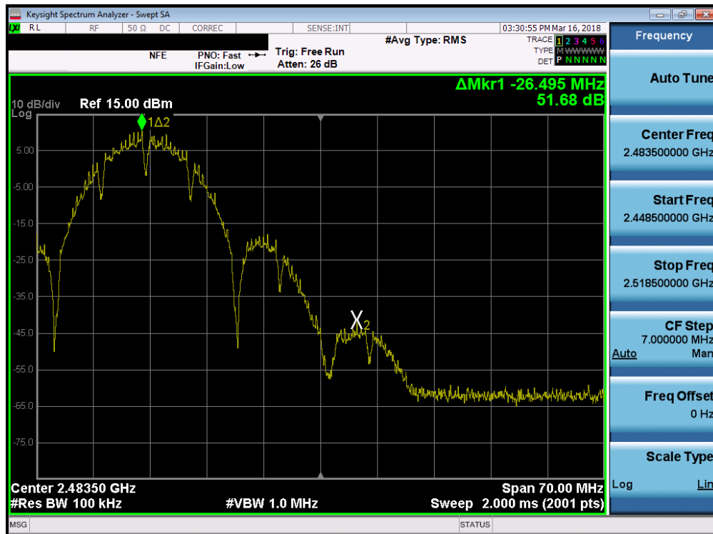
Plot 7-44. Band Edge Plot (802.11b – Ch. 11)
