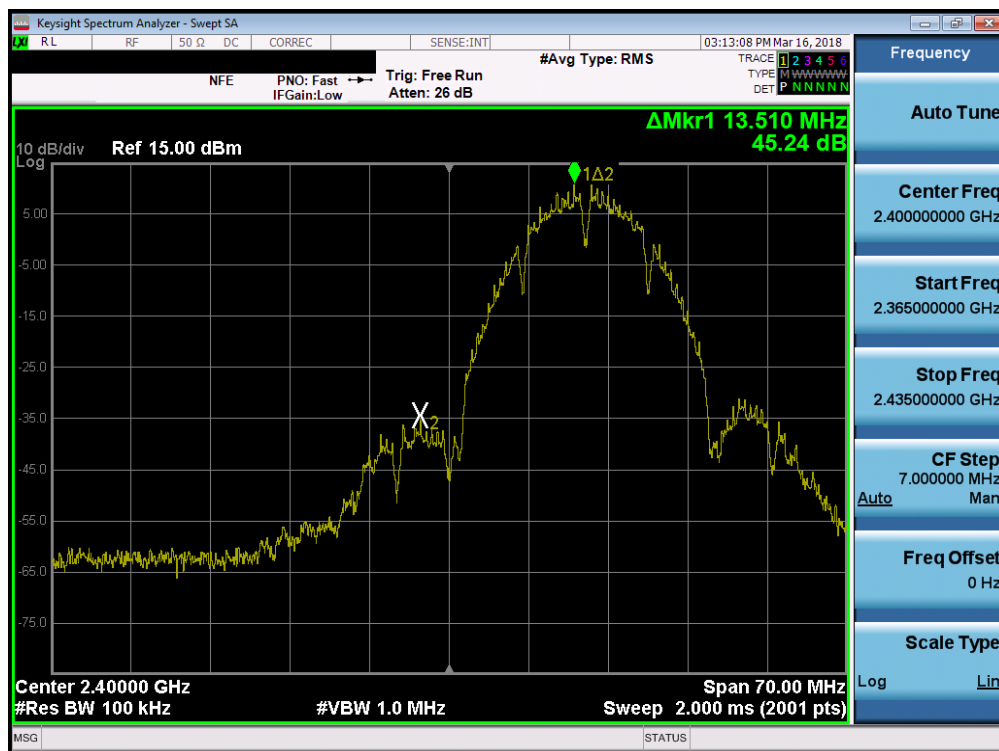
Plot 7-37. Band Edge Plot (802.11b – Ch. 1)
