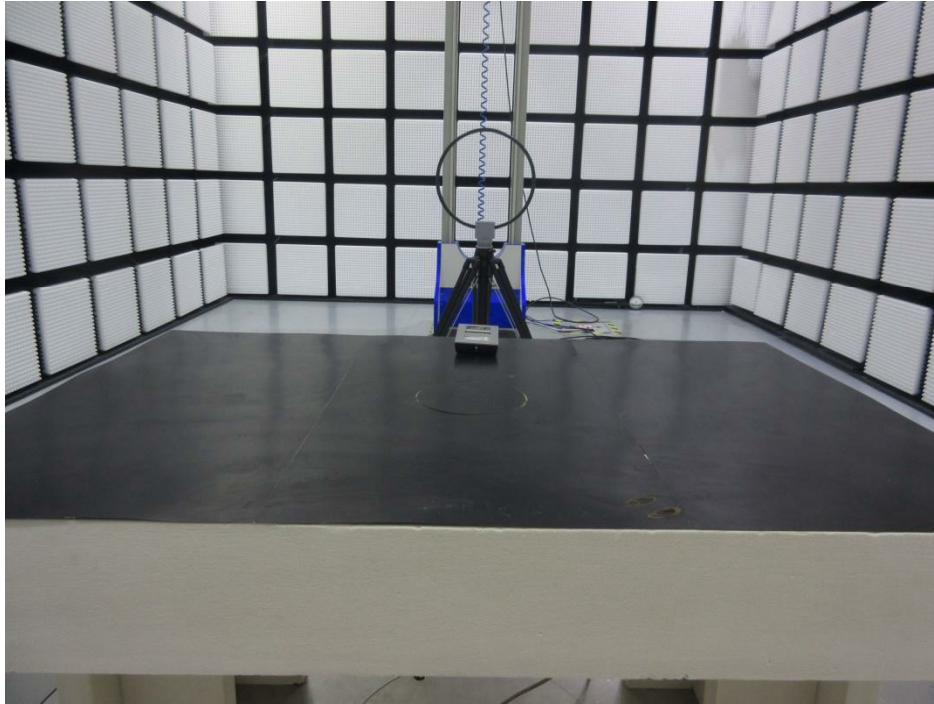
Setup photo of radiated emission (9KHz-30MHz)
