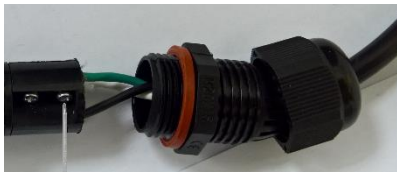
Figure 13: Secure Cable to Connector
