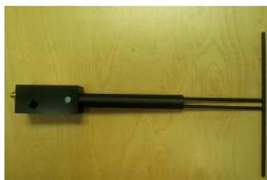
Figure 1 – MVG COMOSAR Validation Dipole
