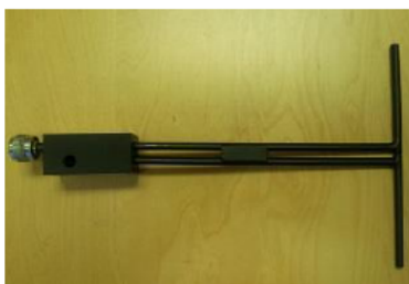
Figure 1 – MVG COMOSAR Validation Dipole
