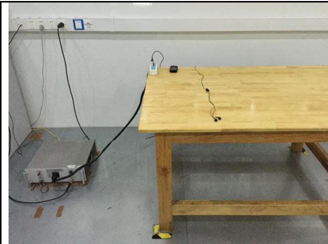
Conducted Emissions Test Setup Front View
