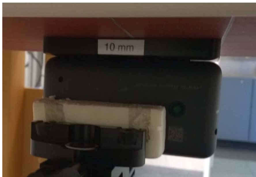
Photo of the device positioned for WR mode measurement – right edge facing phantom. The spacer was removed before the start of the measurements
