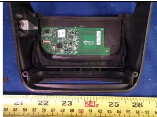
NFC Board Location View
