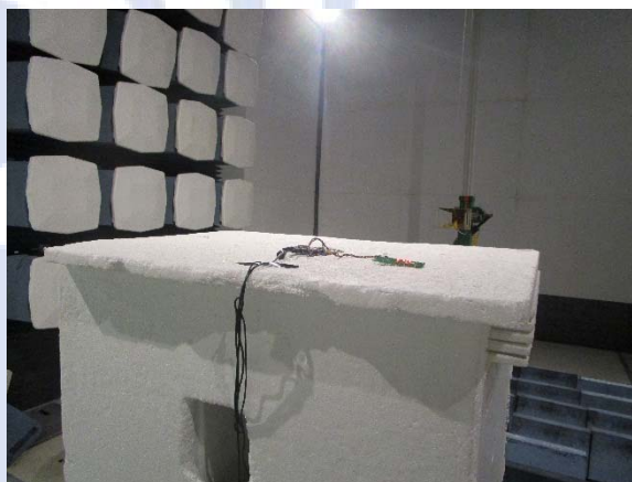
Radiated Emission Test setup (>1GHz) – Rear View
