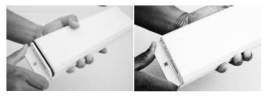
5. Locate the Fastener Bag and remove the two screws. Using a Phillips screwdriver, install the screws to secure the inner housing to the outer housing.
