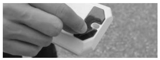
6. Insert the carriage bolt into the holes. To fully seat the fastener into the hole, ensure the square shank of the fastener is aligned with the hole in the module and press the fastener into the ribs. The ribs will help hold the carriage bolt in place and prevent the fastener from turning when the nut is applied to the bolt.
