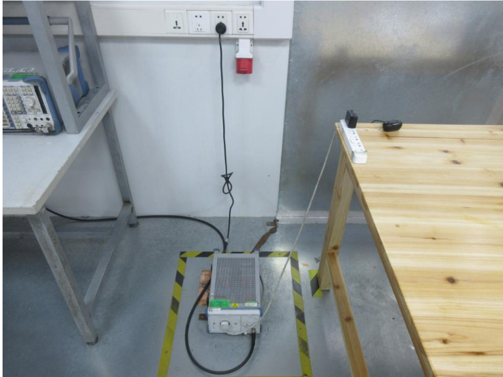
Photo of Conducted Emission Measurement
