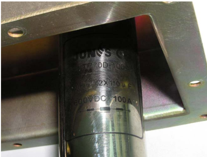
Power Filter Label backup
