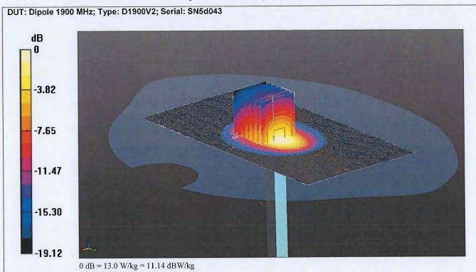
Communication System: UID 0, CW (0); Frequency: 1900 MHz; Duty Cycle: 1:1
