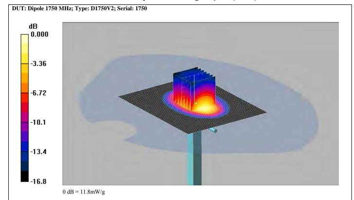
Communication System: CW; Frequency: 1750 MHz; Duty Cycle: 1:1
