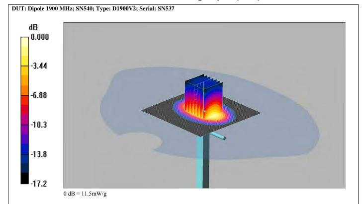
Communication System: CW; Frequency: 1900 MHz; Duty Cycle: 1:1
