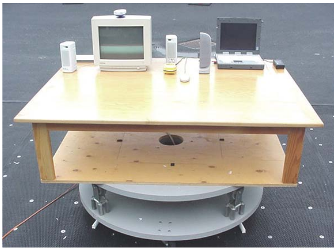
Photograph D-3 - Front of Radiated Emission Configuration
