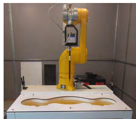
Figure 4.1 DASY5 Test System
