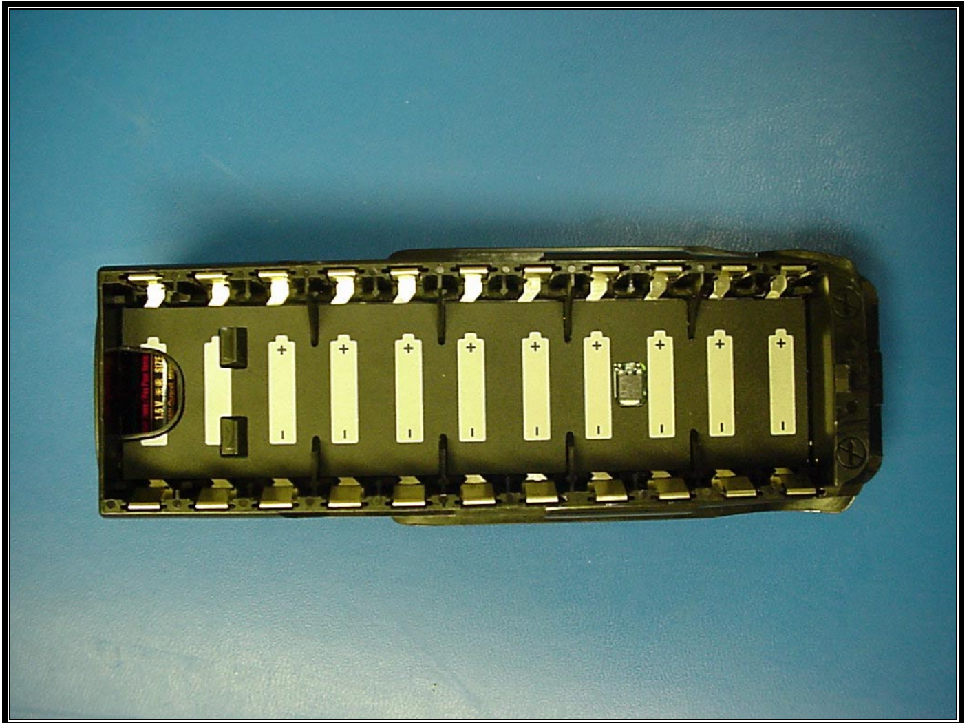
PHOTOGRAPH 8: FRONT VIEW OF BATTERY PACK (CELLS REMOVED)
