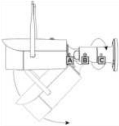
1. Loosen the bolt **C** to swivel the camera so that it is pointing to the direction of the scene desired and then tighten it back.
