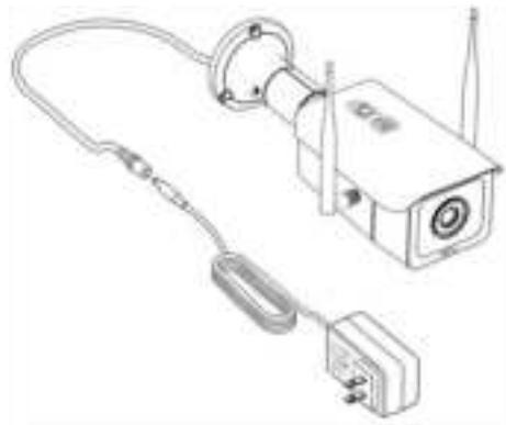
**WARNING:** Do not connect AC power source to the 12V-DC female plug as this will damage the camera and cause fire, electric shock, and other serious hazards. In addition, the product warranty is voided automatically.
