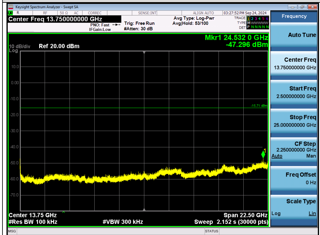
Test_Graph_Custom IEEE 802.11_Chain A_2470_MCS0_Higher Band Emissions
