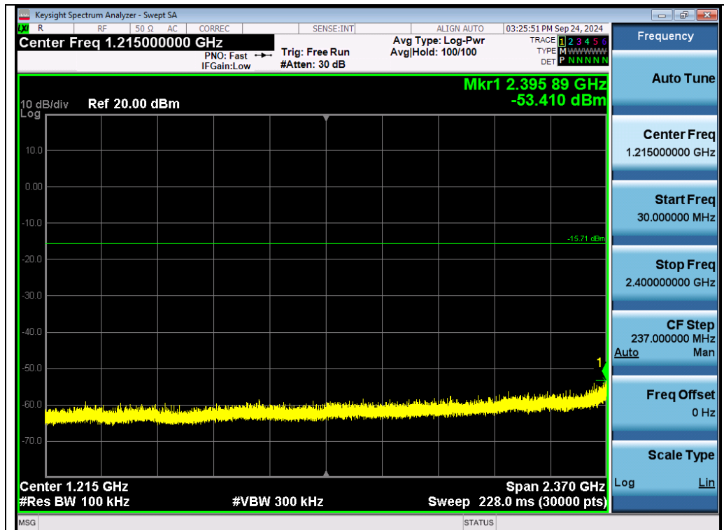
Test_Graph_Custom IEEE 802.11_Chain A_2470_MCS0_Lower Band Emissions
