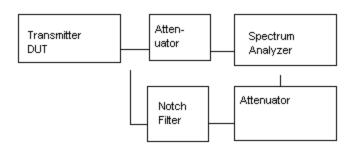
Method of Measuring Conducted Spurious Emissions
