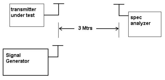
Method of Measuring Radiated Spurious Emissions
