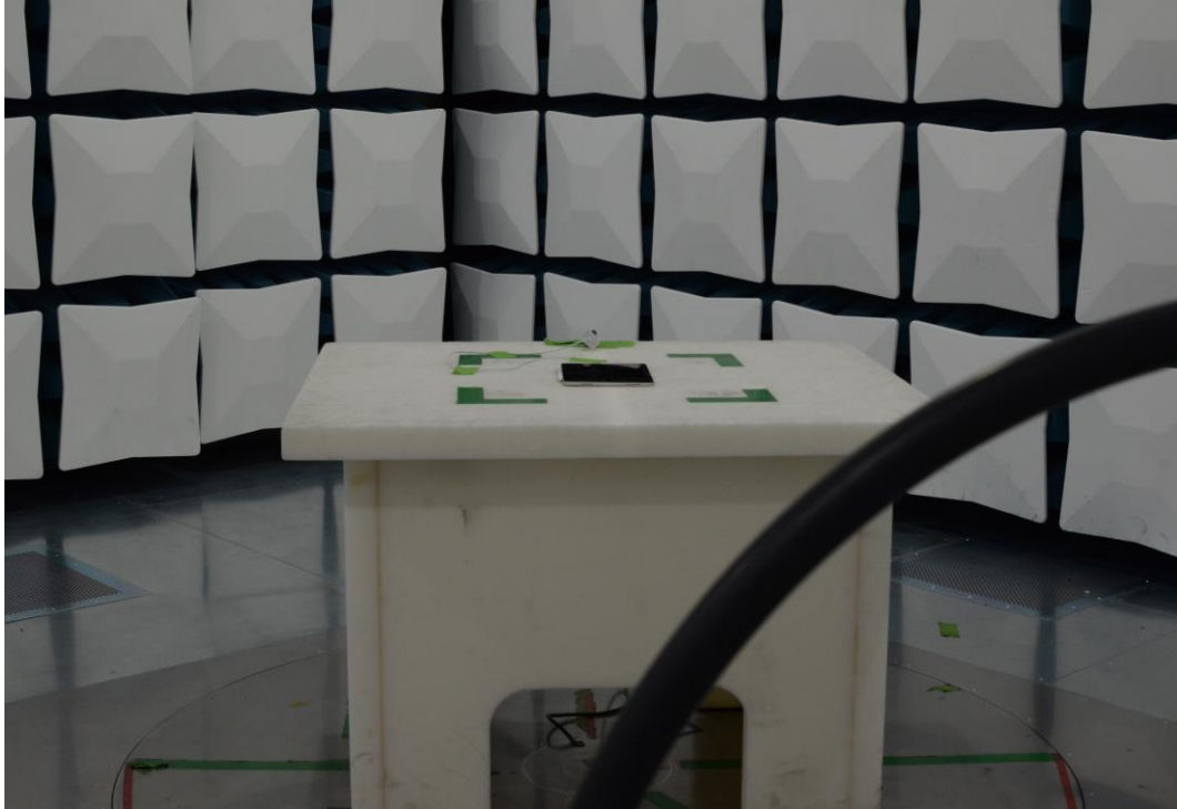
Figure 23: 9kHz-30MHz Test Setup (Front View)
