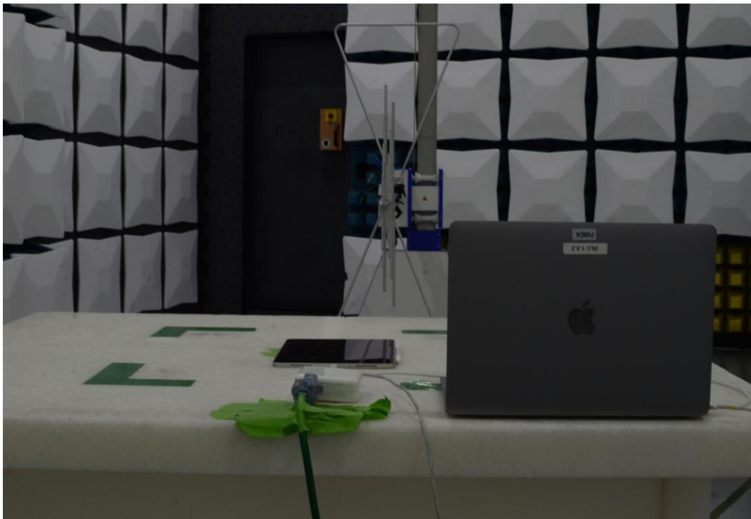
Figure 18: 30MHz-1GHz Test Setup (Rear View)
