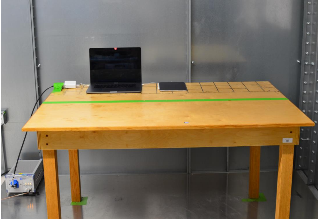
Figure 3: AC Line Conducted Emissions (Front View)
