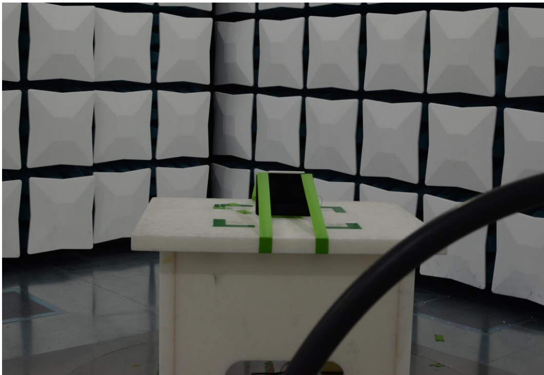
Figure 24: 9kHz-30MHz Test Setup (Front View)
