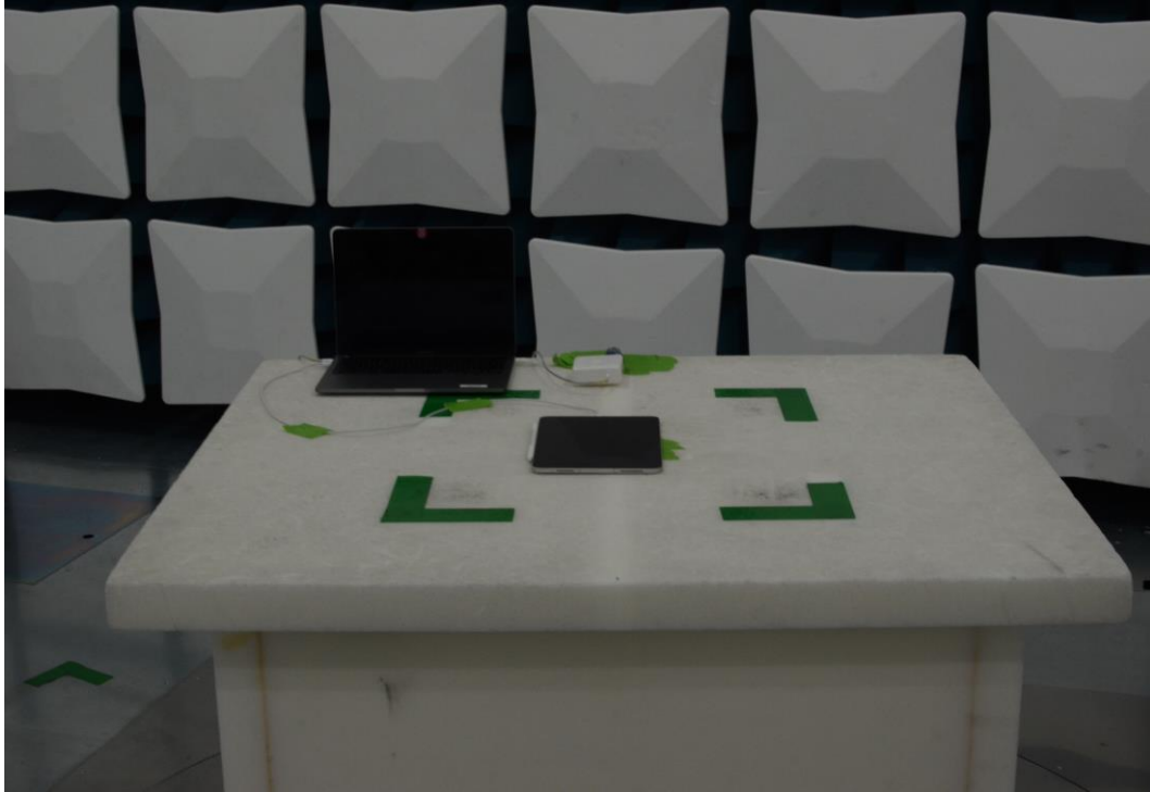
Figure 17: 30MHz-1GHz Test Setup (Front View)
