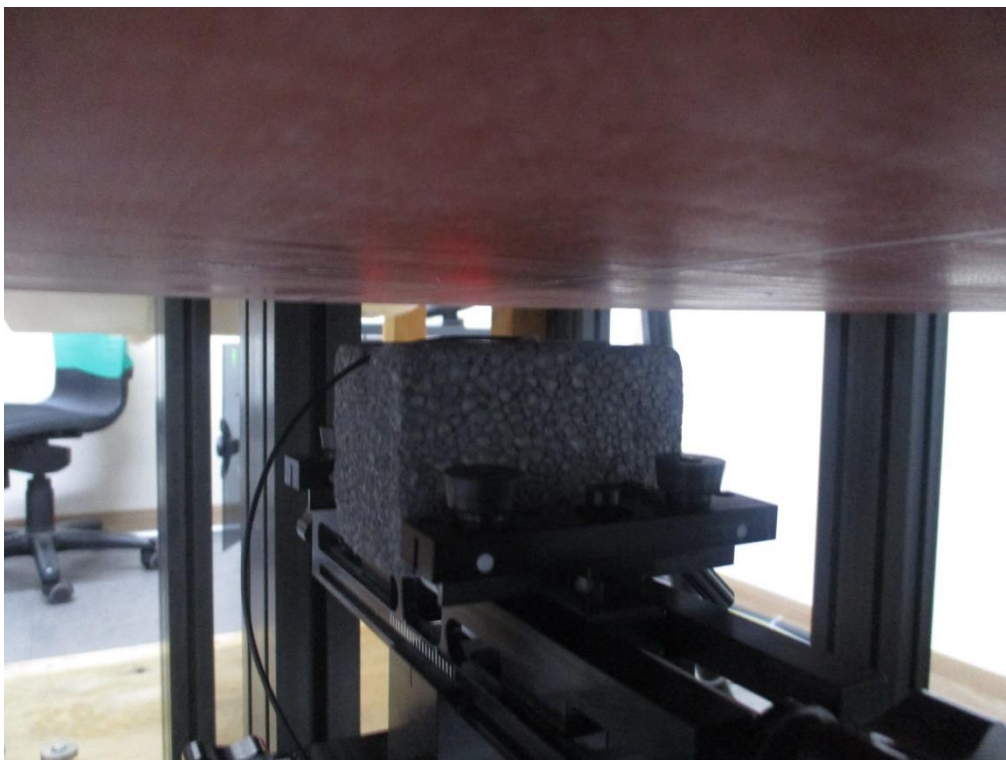
Rear Side from Flat Phantom (Separation Distance: 1.5 cm) – Bluetooth Antenna
