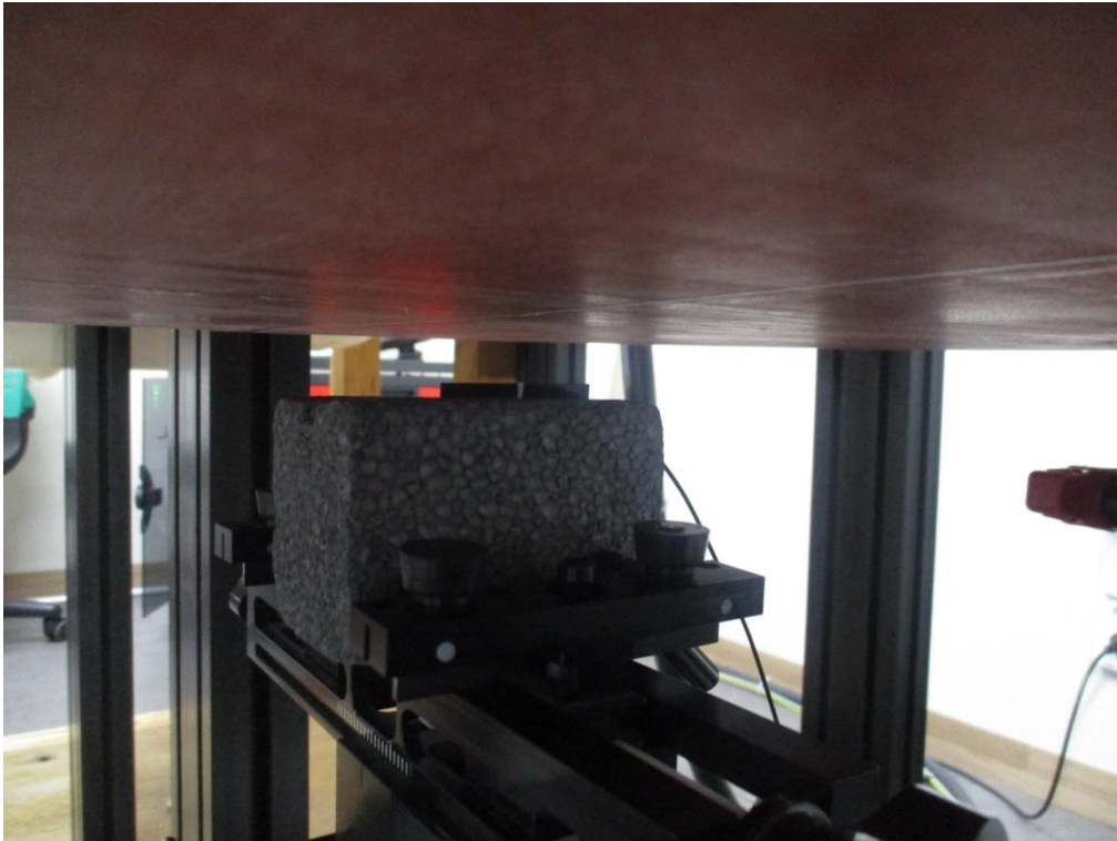
Right Side from Flat Phantom (Separation Distance: 1.5 cm) – Bluetooth Antenna
