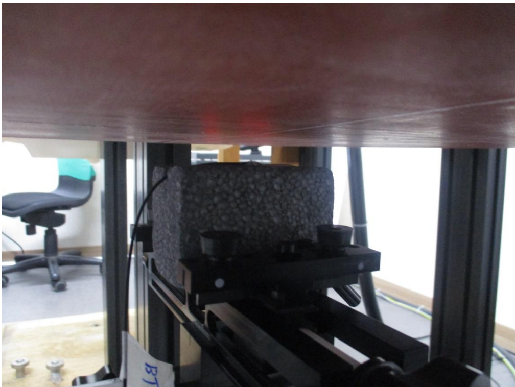
Rear Side from Flat Phantom (Separation Distance: 1.5 cm) – MESH Antenna
