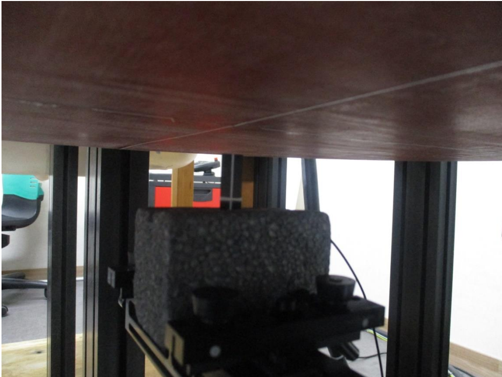
Top Side from Flat Phantom (Separation Distance: 1.5 cm) - Bluetooth Antenna
