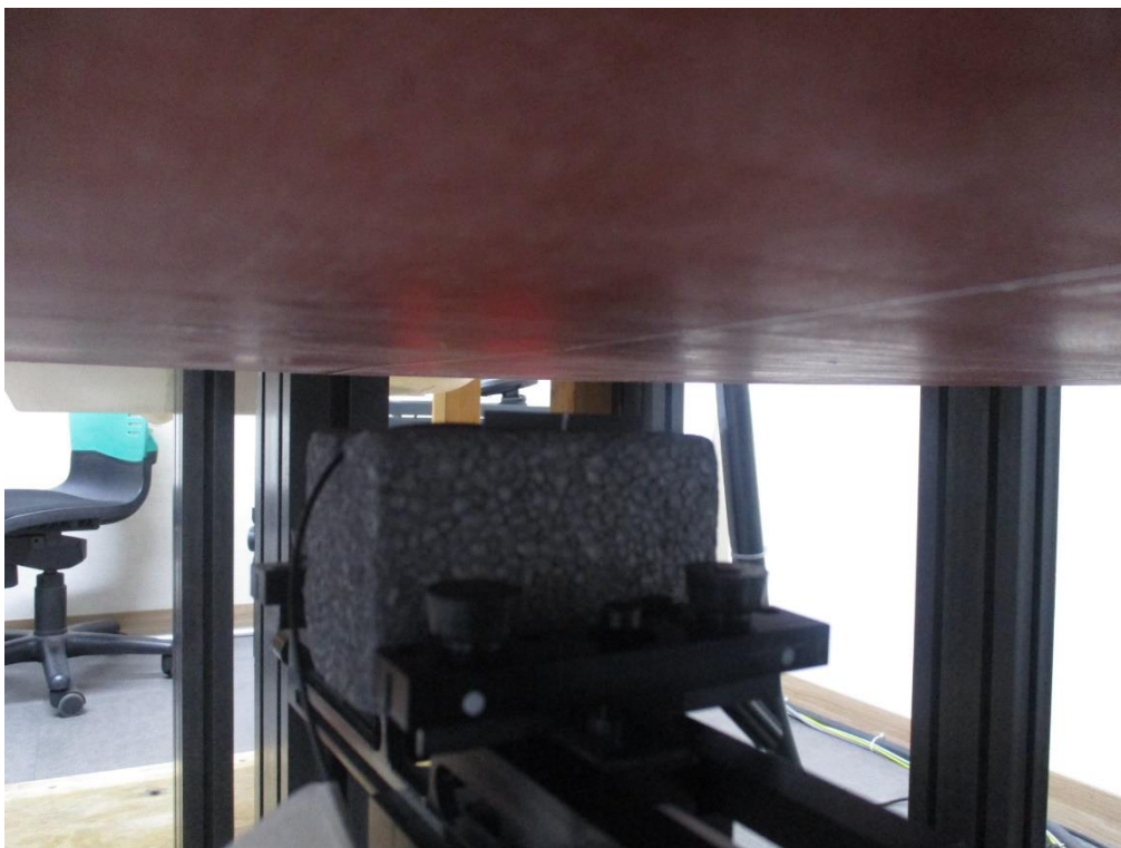
Left Side from Flat Phantom (Separation Distance: 1.5 cm) – MESH Antenna
