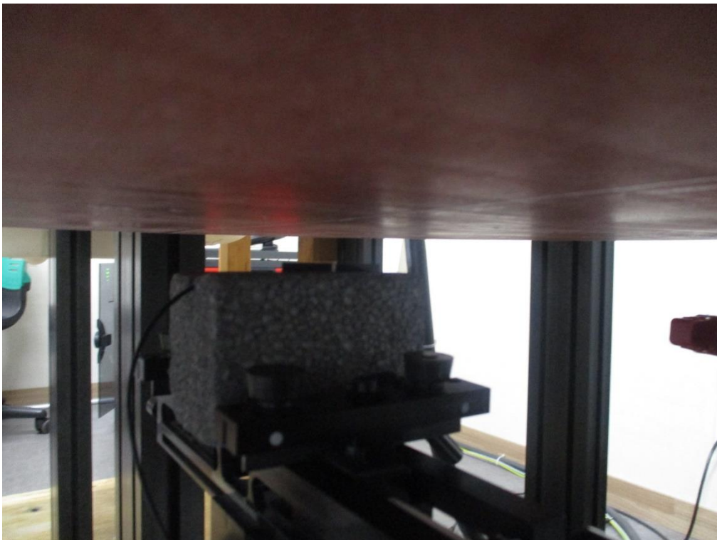
Left Side from Flat Phantom (Separation Distance: 1.5 cm) – Bluetooth Antenna
