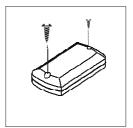
Mount Trackunit Spot using M4 or 5/32 inch screws with minimum length of 2 inches
