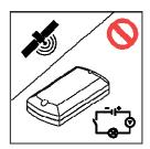
Do NOT install the GPS/(GSM/UMTS) unit directly under a layer of metal or next to wires
