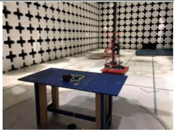
Radiated Emissions (<1GHz) – Rear View
