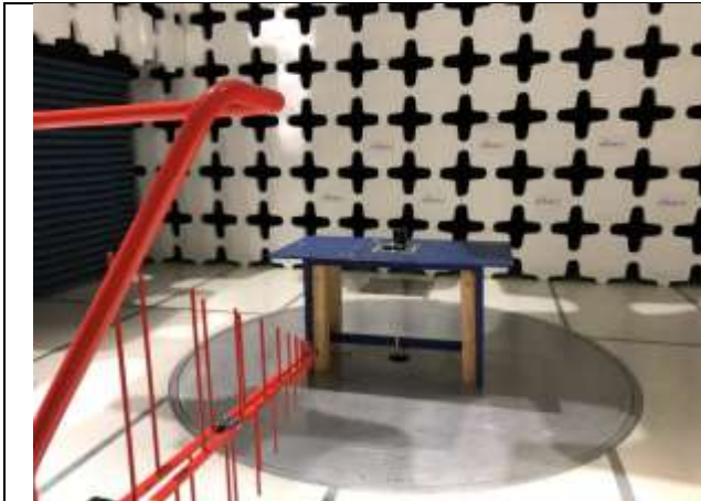
Radiated Emissions (<1GHz) – Front View
