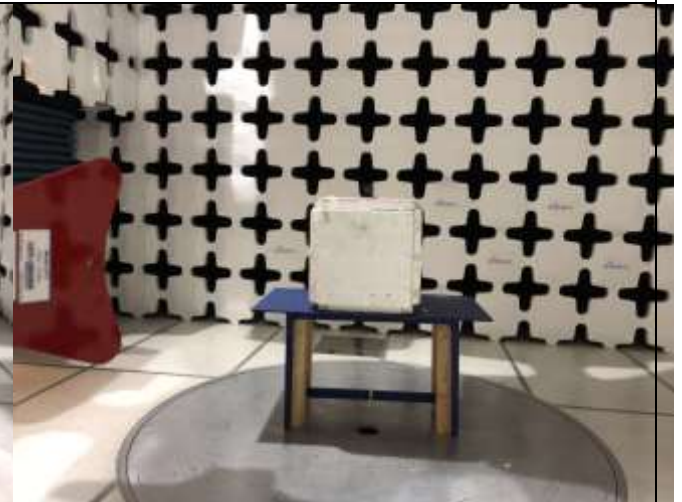
Radiated Emissions (>1GHz) – Rear View
