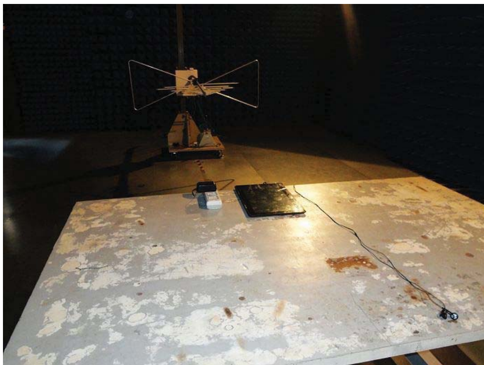
Radiated Emission Test Setup:
