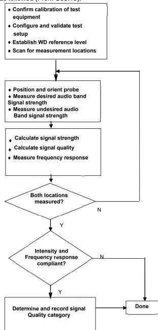
Figure 4-13 **C63.19 T-Coil Signal Test Process**
