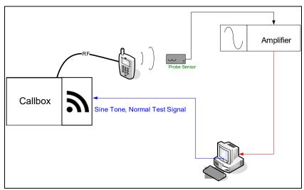
Figure 4-2 T-Coil Test Setup
