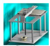
Figure 4-3 RF Near-Field Scanner
