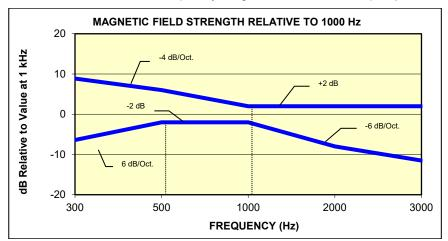
Figure 3-1 Magnetic field frequency response for Wireless Devices with an axial field ≤-15 dB(A/m) at 1 kHz
