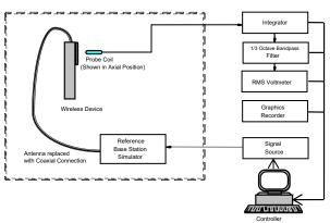
Figure 4-12 **Audio Magnetic Field Test Setup**
