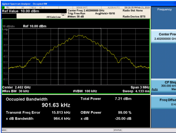
20dB Bandwidth plot on channel 39 (1Mbps)
