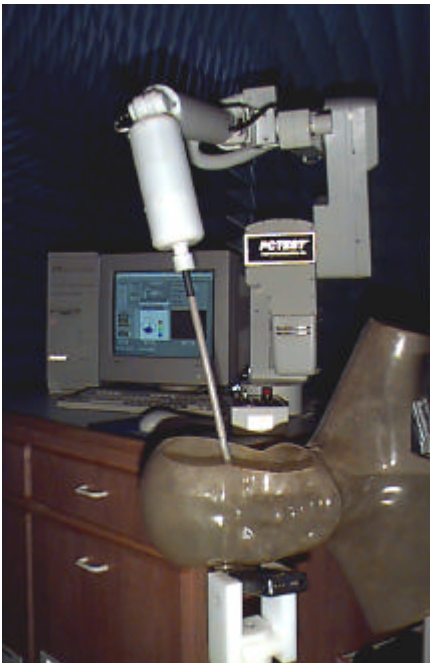
Figure 5. Photograph of the Probe and the Phantom
