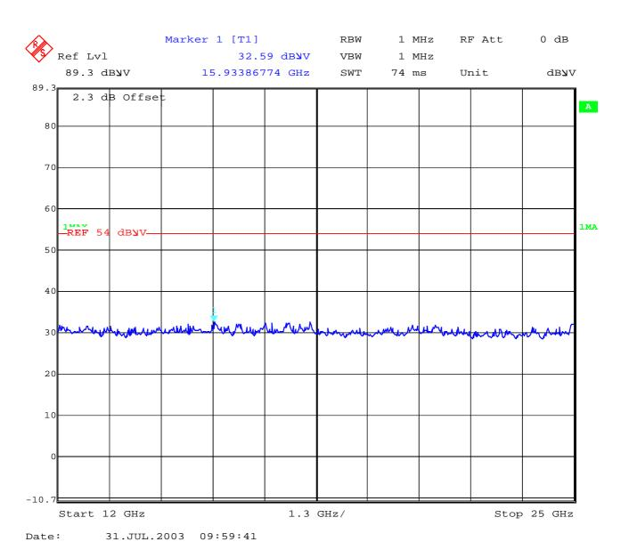
For this measurement we used a special wideband horn antenna and a low noise preamp.
