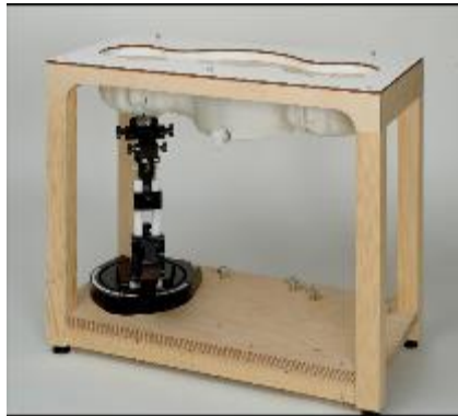
Picture C.10: SAM Twin Phantom
